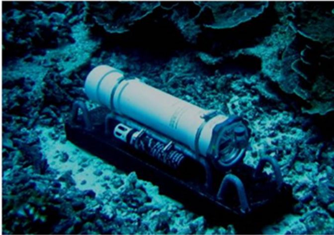
Figure 4.12. Environmental Acoustic Reader (EAR) in a coral reef (source: M. Lammers)
