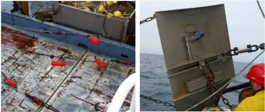
Figure 3.29. On the left: tensionsensors on the bracket of an experimental trawl, positioning system, system used to measure distance between the otter doors and their depth, otter door angle sensor (vertical cylinder). On the right: acoustic beacons working as master-slave to measure the horizontal opening of a pelagic trawl in relation to its rigging (source Ifremer – [VIN 08, VAC 04])
