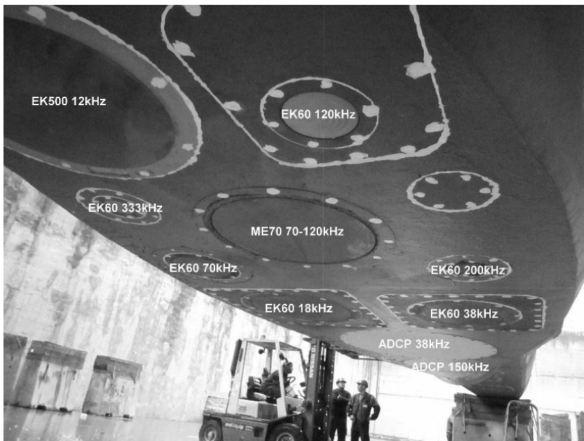
Figure 4.9. Echosounders installed on the hull of RV Thalassa (source: Ifremer)
