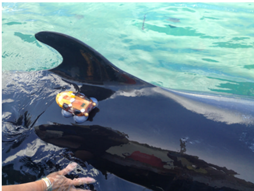
Figure 4.13. Digital Acoustic Recording Tag (DTAG) on an Atlantic bottlenose dolphin ( Tursiops truncatus ) (source: Aliza Millette – Winfree)
