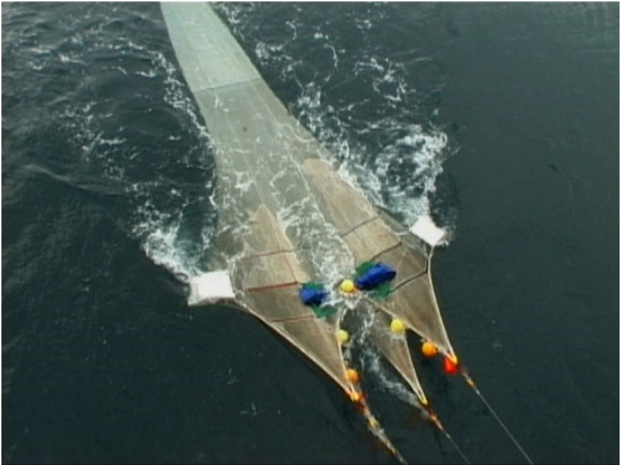
Figure 3.13. A “mesopelagos” scientific trawl (source: Ifremer – M. Meillat)
