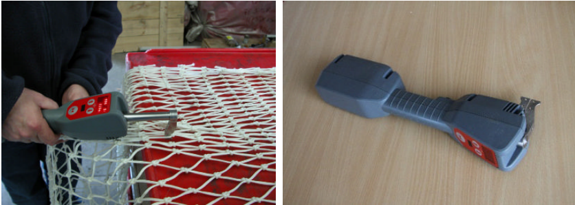
Figure 3.5. The OMEGA gauge (source: Ifremer/G. Bavouzet – P. Larnaud)
