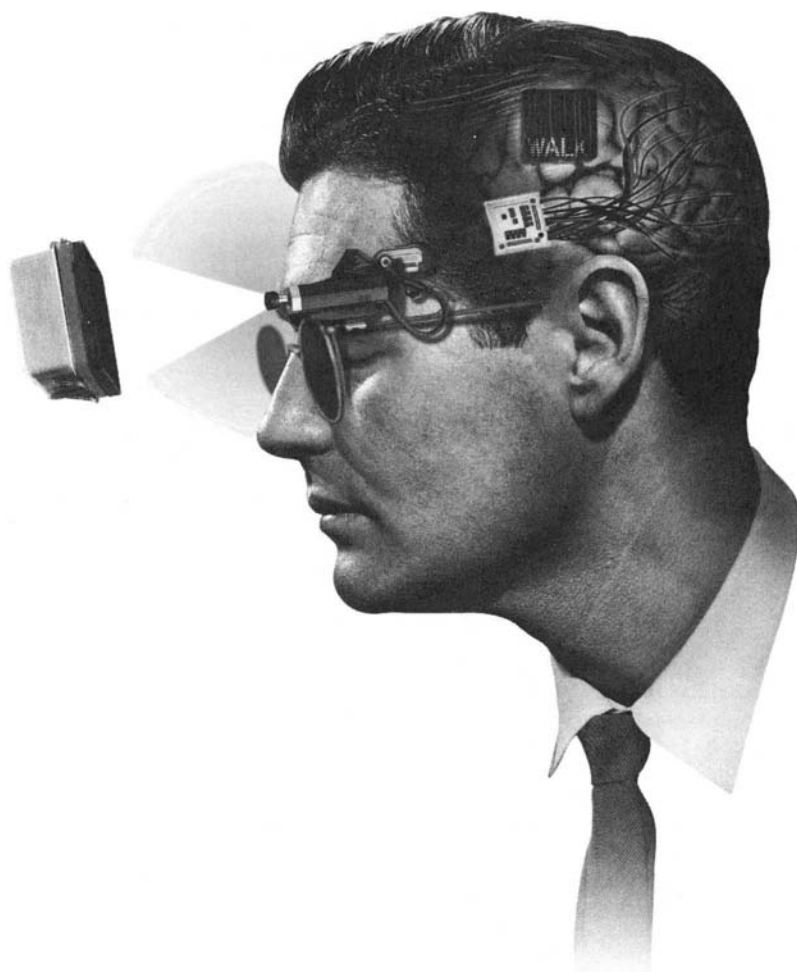
FIGURE 1.33. Concept of an intracortical visual prosthesis. The camera captures the image and translates the visual information into stimulation sequences. Transcutaneous power and data are sent to the implant over a common inductive link. (Courtesy of Illinois Institute of Technology)
