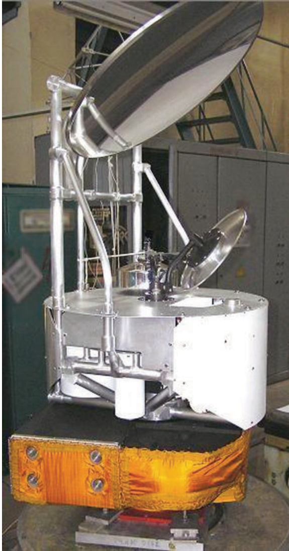
Fig. 5.3 Microwave scanner/sounder MTVZA GY
