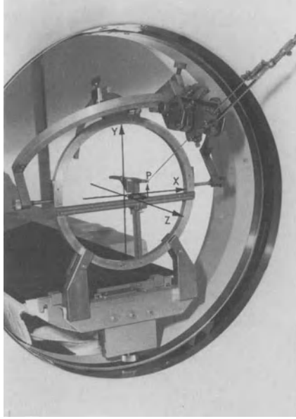
Fig. 1. Presentation of the CT scanner gantry with the stereotaxic device developed by Riechert and Munding in the computer compatible modification by Munding and Birg. The cartesian target point coordinates of the stereotaxic device are identical with the coordinates of the CT scanner when the 0-point of the stereotaxic device is in the origin of the CT scanner
