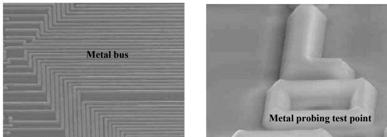
Fig. 23.13. Metal bus. A signal bus realized of metal can be recognized on the left, note that the curvature of the angles is the same for all the metals. On the left a test pad, realized by means of a metal ring as to easily insert the microprobes used during laboratory analyses
