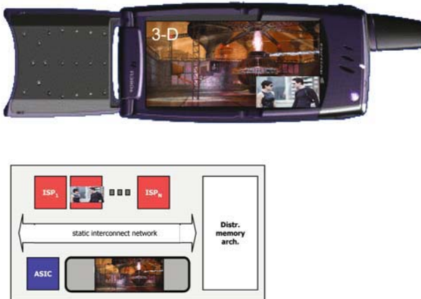
Figure 2-13. A 3D application is running on the reconfigurable hardware, while the video application continues in a reduced window and on a software processor
