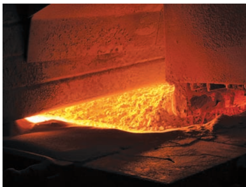
Figure 2 “Batch” is a mixture of very high-quality silica sand and other materials such as salt cake, limestone, dolomite, feldspar, soda ash, and powdered cullet. Glass is made by melting and cooling the batch. Source: From Ref. 9, with permission from Elsevier.
