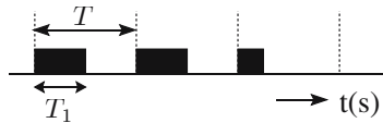
Figure 4-7. Stretch of the response time of an actor due to preemption in the case that the actor starts at the begin of interval T_1 .
