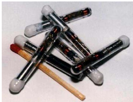
Figure 2.7: Photograph of a few injectable transponder prototypes.
