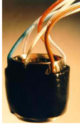
Figure 3.8: Brånemark abutment equipped with 3 strain gauges.
