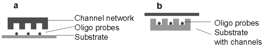
Fig. 7.2. Evolution of the fabrication process for biochannel devices, (a) oligo probes are spotted on the flat surface and overlaid with PDMS channel network, (b) oligo probes are spotted into the channels directly and overlaid with flat cover piece
