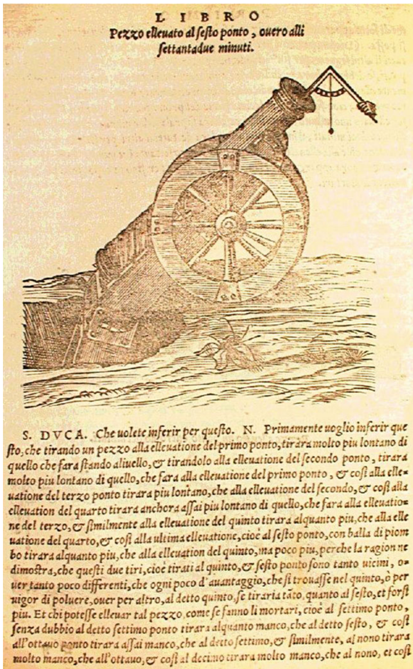
Fig. 1.17 Plate from Quesiti on inclined cannon for the maximum path and bombardier's quadrant (Tartaglia 1554, Book I , Q I, 6v; Ivi , Q I, 5rv-7rv)
