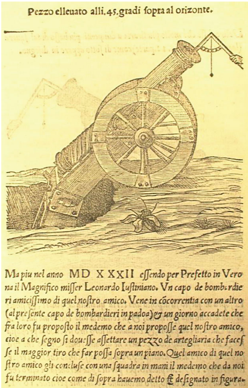
Fig. 1.15 Plate from Nova scientia around 45-degree elevation and bombardier's quadrant (Tartaglia 1537, 4r; as above cited, in Nova scientia Tartaglia canonically enounces his fundamental theorem (as general law) about 45-degree (Tartaglia 1537, Book II , Pr. VIII, 28v). We take this opportunity to remark – in our opinion and strictly based on original Tartaglia's reasoning both Nova scientia and Quesiti – an overstress in the secondary literature concerning an assumption according to which Tartaglia discovered – as a corollary – that ranges are equals for elevations as 45^\circ \pm \gamma . Of course, Tartaglia never wrote about that in his works. Tartaglia only discussed – without any physics-mathematical relation – on the possibility that a certain target can be fired by two different heights/elevations. An eloquent image is reported in Quesiti (Tartaglia 1554, Book II , 7v). This is different from the assumption that particular physical and technical conditions (i.e., dimension and weight of cannonball, equipment, etc.) allow to fire two subsequent shots so that initial velocities of the projectiles, in practice, have the same value)
