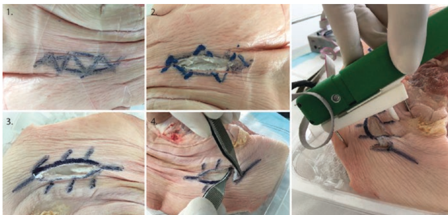
Fig. 7.2 Wound tension testing of zigzags and Z-plasties on pigskin
