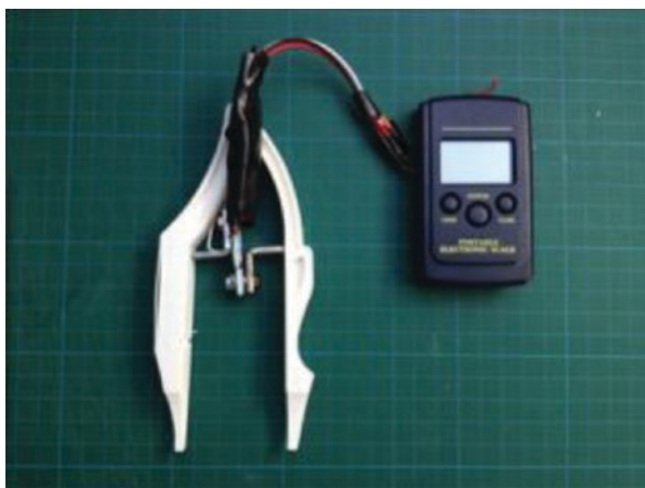
Fig. 4.2 Initial prototype was shaped like forceps, but needed modification of design
