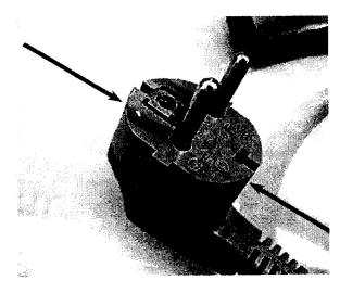
**Plate 4** A European plug. The item has nine internationally recognized safety approvals. If the Safety Earth Ground corresponding socket has an earth 'PIN', then this plug is polarized. If the Safety Earth Ground connection is made via the arrowed contacts, then this plug is not-polarized. Therefore short-circuit protection between Neutral and Ground must be investigated and provided
