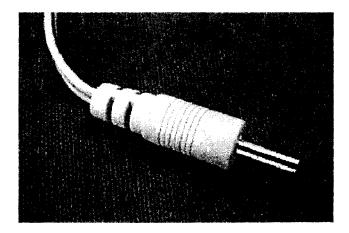
**Plate 20** In product safety terms this type of connector is identical to the illustration in Plate 19 as the electrical connections are 'operator' accessible. The power is less than the maximum level defined by the Safety Extra Low Voltage Energy Limited requirement of the relevant standard – this is specified as 15 W maximum in several standards
