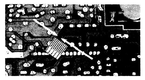
**Plate 11** Showing a power supply unit (PSU) that has basic insulation between hazardous and SELV circuits. This choice of PSU will, most likely, increase the amount of abnormal testing significantly
