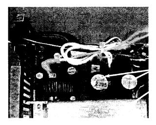
**Plate 2** Problem: the light-grey wire is rated 300 V and supplies the fan from SELV circuitry. This basic insulation does not provide adequate protection from the hazardous voltage on the bare metal of the mains socket; the capacitors are charged at up to 360 V peak and are storing 31 J; or the unearthed heat sink. Solution: fit supplementary insulation over the fan lead. Use wire with reinforced insulation (greater than 0.4 mm thick)
