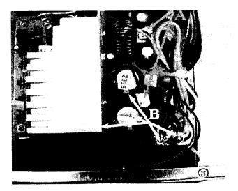
**Plate 3** Problem: the connector 'A' fitted to the end of this flying lead is not physically retained with a clip. Once detached (a single fault) the flying lead can contact various hazardous parts 'B'. Solution: use a connector with an indent, or use cable tie or tie wrap to limit movement of flying lead, when it is unplugged
