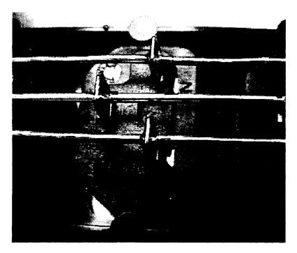
**Plate 16** These connections are 'daisy-chained' but because a single strand of wire is used the connections can be considered 'reliable' since if one solder joint fails the wire cannot move or break contact
