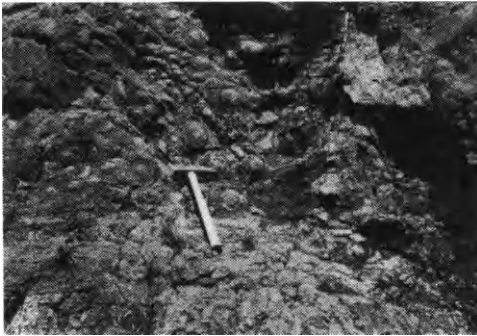
Figure 7.1b Spheroidal weathering of basalt lava flows, Tideswell, Derbyshire. In places these lavas are completely decomposed
