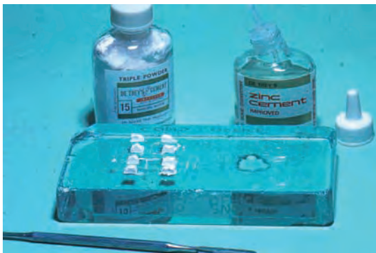
Fig. 28.1 A zinc phosphate cement supplied as a white powder containing primarily zinc oxide and a colourless liquid which is an aqueous solution of phosphoric acid. Mixing typically is performed on a glass mixing slab of the type shown.
