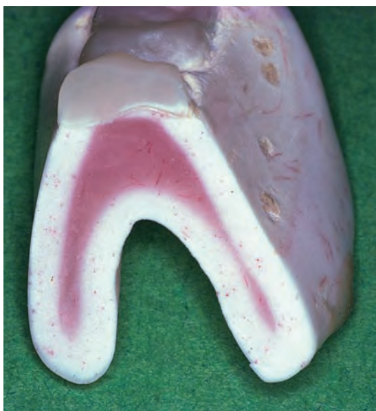
Fig. 13.11 Whitened denture base. This shows a section through a denture base which has been whitened by the patient using an oxygenating cleanser in hot water ( >90^{\circ}\text{C} ). The original colour of the denture can be seen in the middle of the section and we can see that the whitening effect has progressed inwards from the outside surface. The original pink colouration of the veins which are present in this material can also be seen.
