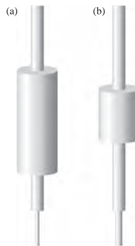
Fig. 3.3 Indentors used to assess setting characteristics of gypsum products. Sometimes referred to as Gilmore needles. Ability of support needle (b) indicates the initial set. Ability to support needle (a) indicates final set.
