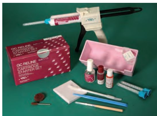
Fig. 14.4 A silicone denture soft lining material. The type of silicone used here is an addition curing product. It is provided in the form of a cartridge containing two pastes which are mixed when the pastes are extruded through the nozzle. The other items shown are those which are required to achieve bonding of the silicone to the acrylic denture base, for trimming the soft lining material and for coating the soft lining material after setting.
