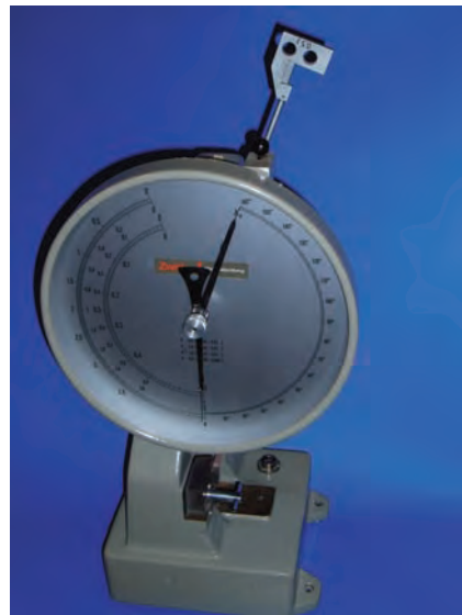
Fig. 2.8 Test equipment for the Charpy impact test. This shows the equipment used to determine impact strength. The essential part of this equipment consists of a pendulum which swings from the position shown, down and then up again to the equivalent position on the other side. If a specimen is located at the bottom of the swing, as the pendulum swings through, it fractures the specimen and as energy will be absorbed in this process the pendulum swings up to a lower position on the other side. Hence, the energy absorbed in fracturing the specimen is shown on the gauge. Since this equipment gives a direct measure of energy absorbed during fracture this is strictly speaking a measurement of toughness rather than strength.
