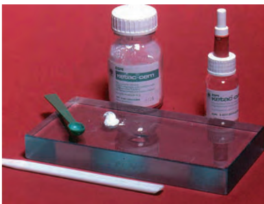
Fig. 30.3 A glass ionomer lining and luting cement. The material is provided as a powder and liquid which are mixed together on a mixing pad or on a glass slab as shown. The material is chemically similar to the glass ionomer cements used for restorative purposes. However, the luting cements are formulated to produce a cement with lower viscosity which will flow to form a thin film.
