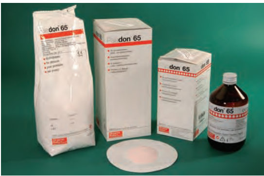
Fig. 13.2 Denture base acrylic. This shows a typical acrylic denture base material which is provided in the form of a powder (normally containing a pigment which is pink) and a liquid which is contained within a light-proof dark brown bottle. During use the powder and liquid are mixed together to form a dough, which can be moulded inside a mould produced from a cast of the patient's mouth.
