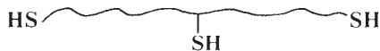
Fig. 19.2 Simplified structural formula of the polysulphide prepolymer showing terminal and pendant –SH groups.
