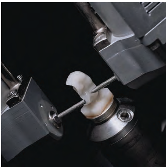
Fig. 11.4 Milling of CAD–CAM restorations. Here we see the milling operation in progress. We can see that the blank has already been cut near to the final shape and following the completion of this process the dental restoration will be removed from the machine and will be ready to be cemented into the patient’s mouth. Figure reproduced with permission of www.planetcerec.com .
