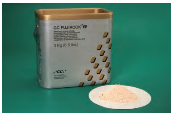
Fig. 3.2 Dental stone. This shows powdered dental stone which is a gypsum product commonly used in dentistry for making casts and models. Note the colour of the stone which in this case is pale yellow. This is to enable the user to distinguish it from dental plaster which although chemically similar is of a different physical nature and is normally white coloured. In use, the powder is mixed with water to form a paste which then hardens to form a hard mass.
