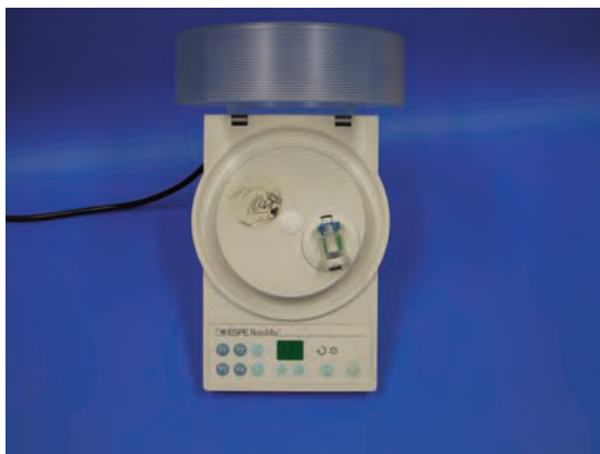
Fig. 24.4 A rotary mixing device which can be used as an alternative to the shaking device shown in Fig. 24.3. In this instrument the capsule is rapidly rotated and centrifuged and the aim is to attempt to produce a mix which contains lower levels of porosity.
