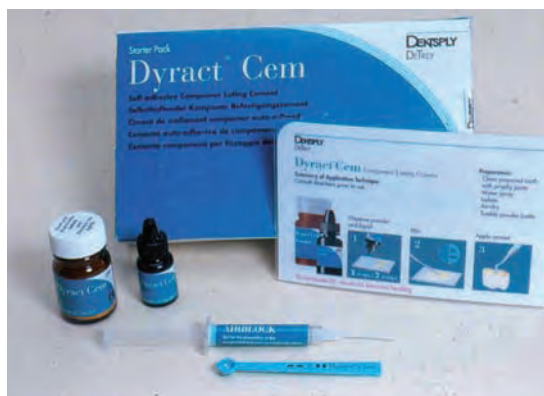
Fig. 30.6 A compomer-type luting cement. The material is provided in the form of a powder and liquid which are mixed together on a mixing pad. The initial setting reaction involves polymerisation and for this type of cement the reaction is strongly inhibited by air; therefore the manufacturer provides an air-block gel which can be seen in the syringe at the front of the photograph. The air-block gel is applied over the exposed surfaces of the cement to ensure that the cement can polymerise correctly.
