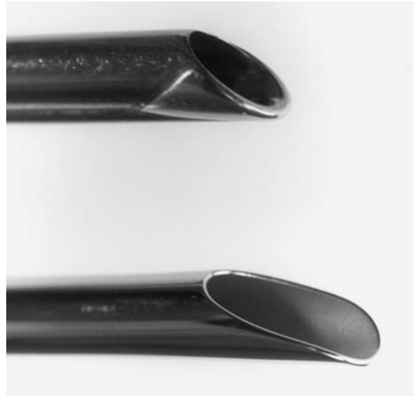
FIGURE 5-3 Comparative tips of Jackson (above) and Storz (below) rigid bronchoscopes. The Jackson model is more easily introduced into a tightly stenotic lesion with a rotatory motion than the Storz model, with its more shovel-like tip.
