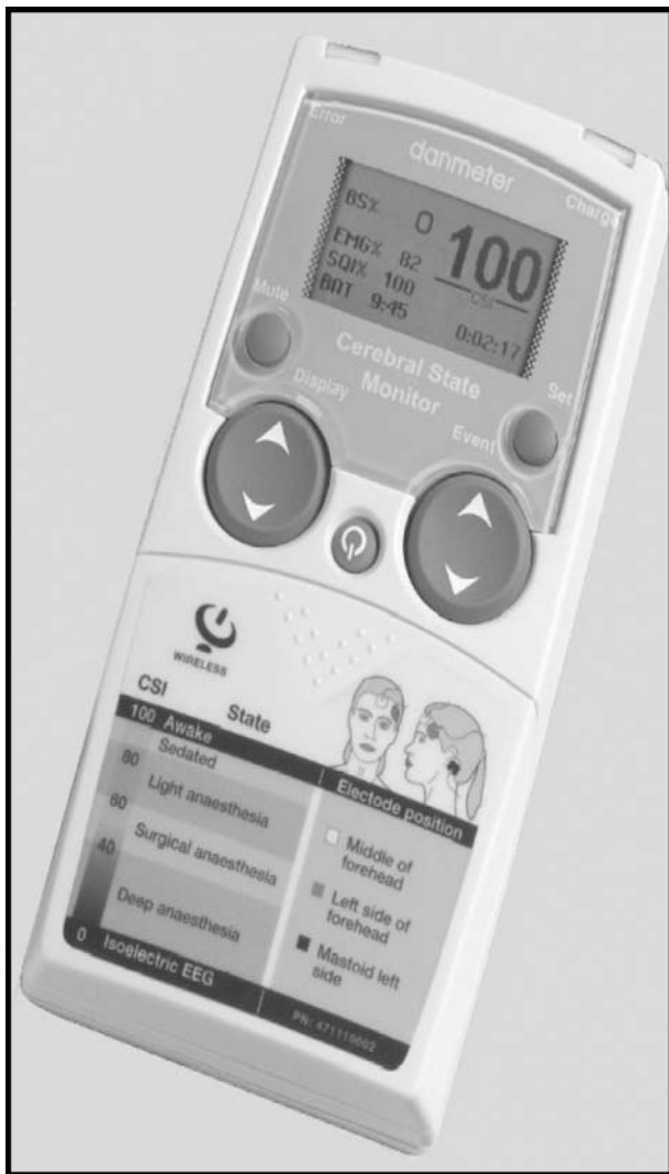
Fig. 92. The handheld ultralight (150g) cerebral state monitor (60 × 117 mm) determining the patients state of unconsciousness.
