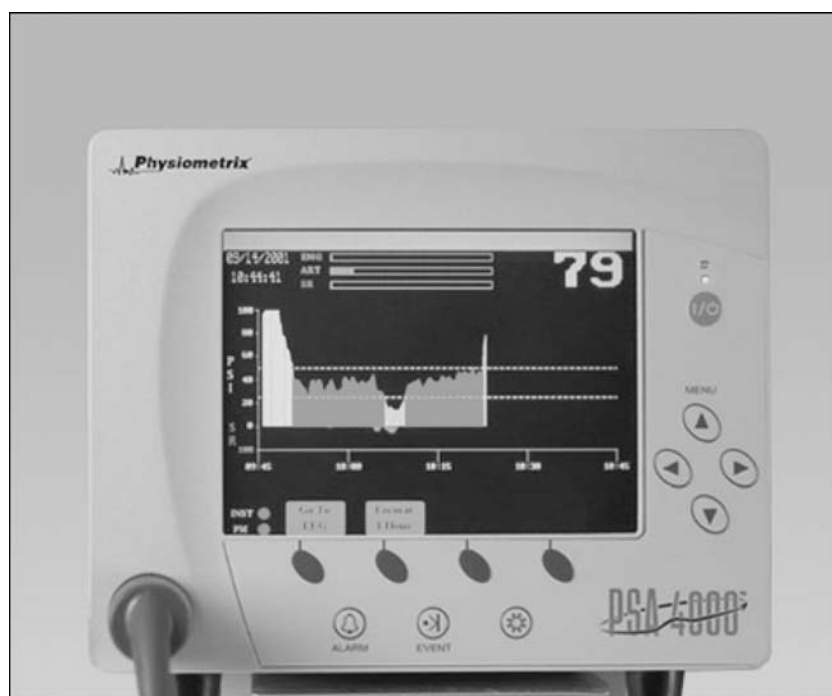
Fig. 84. Front view of the PSA 4000 EEG monitor with the integrated patient state index (PSI) in a numeric form.
