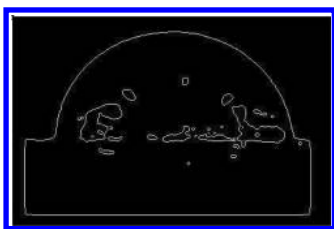
Figure 4. Droplet boundary detected in Canny method.
