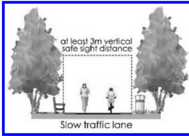
Figure 7. Section of transformation of greenway.
