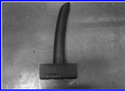
Figure 10. Sub insert from DMLS process.
