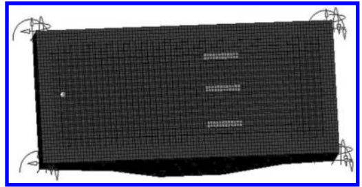
Figure 3. The simulation model of the model car with particle dampers.
