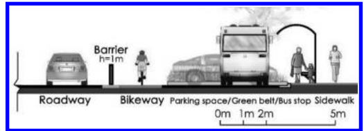
Figure 5. Section of transformation of Datong Road.
