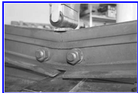
Figure 7. Deformed rail and rail joint after the experiment.
