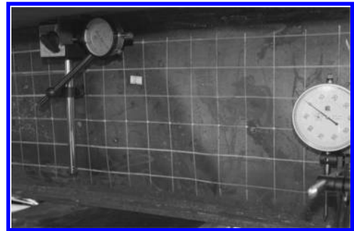
Figure 6. PSCB1-1 local buckling.
