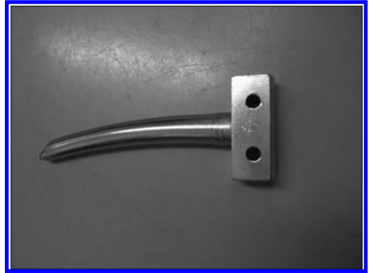
Figure 3. Sub insert for rinsing spray injection mold.
