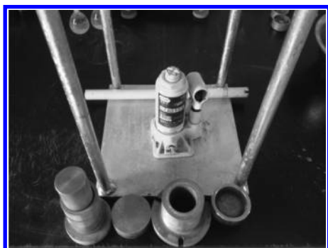
(b) Sample preparation of remolded soil
