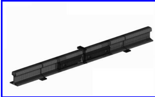
Figure 4. FEM calculation model a detail of a mesh in a rail and rail joint.
