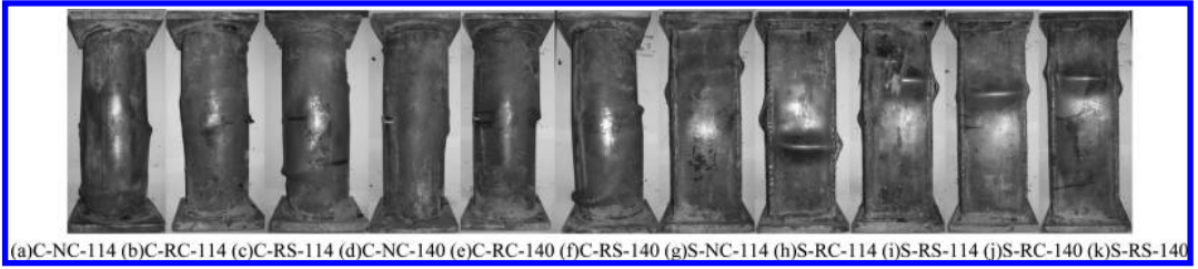
Figure 2. Failure modes of specimens.
