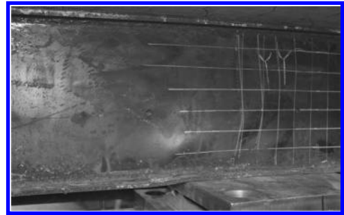
Figure 5. PSCB1-1 local buckling.
