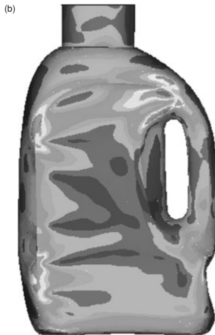
Figure 11.7. (a) Top load test and (b) analysis contour plot.
