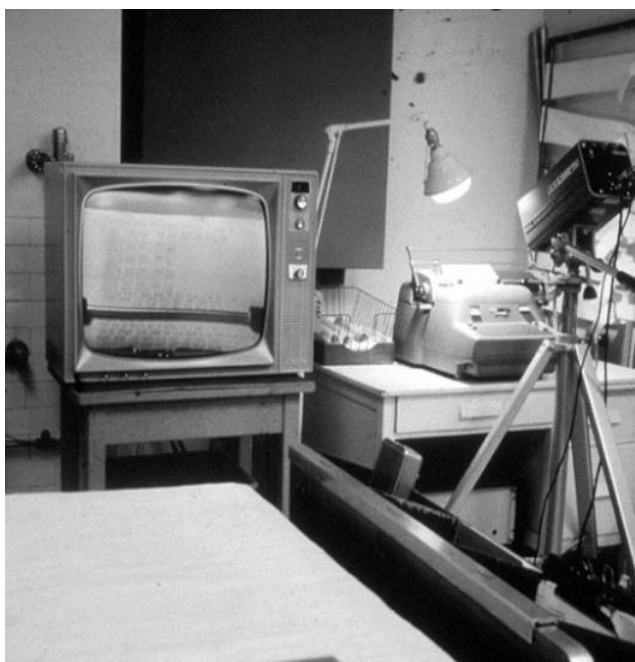
Fig. 1.3 Closed circuit TV camera to project printout from teletype to a TV monitor above the bed, University of Southern California
