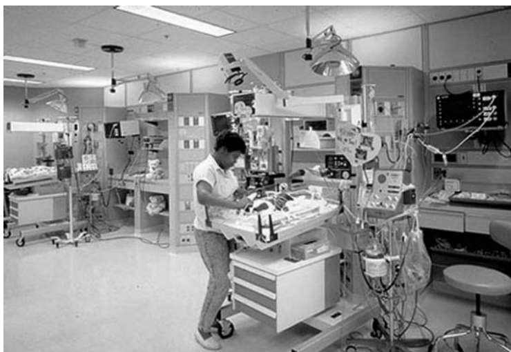
Fig. 40.2 A contemporary space with pendant-mounted services, natural light, windows to the corridor, wooden paneling to soften the space
