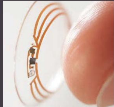
Google is developing a contact lens that senses blood sugar by analysing tears
