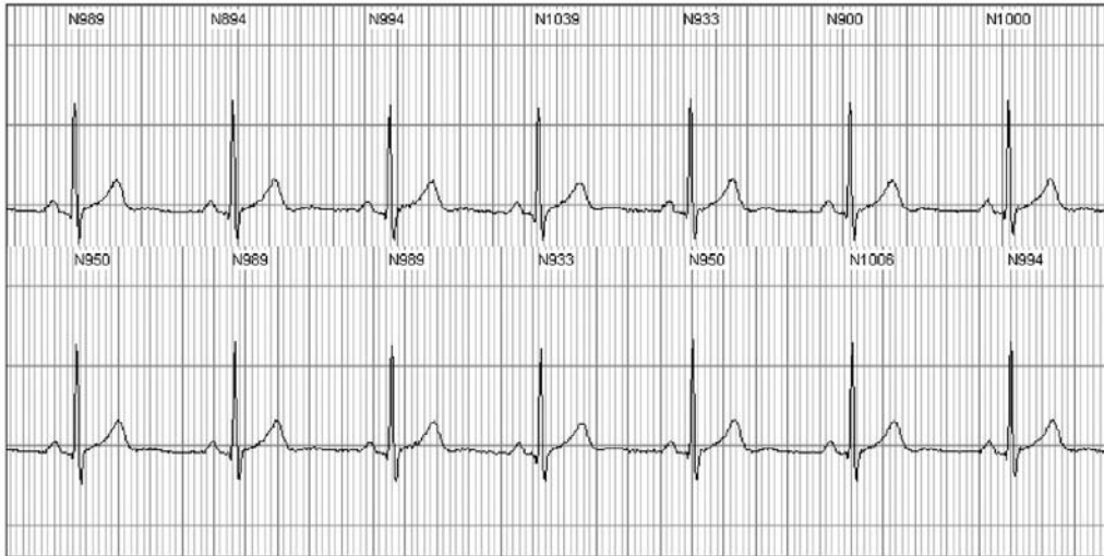
Fig. 4. ECG strip shown before (upper panel) and after (lower panel) jitter correction. Before correction, the positioning of beat labels fluctuates from one beat to another whereas after correction they are stabilized. Even the RR interval sequence is seriously affected with changes up to 100 ms long.
