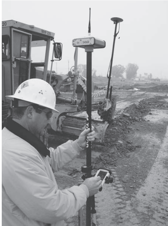
Figure 15.7 GNSS antenna mounted on a grader blade. (Courtesy Topcon Positioning Systems.)
