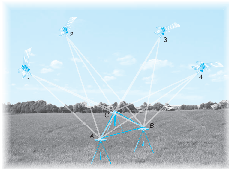
Figure 14.7 GNSS observation session using three receivers. In the case shown, AB and BC are considered nontrivial baselines. Thus, AC is a trivial baseline.
