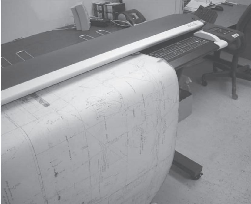
Figure 28.9 Large-format scanner. (Courtesy of Office of Surface Mining, Reclamation and Enforcement, National Mine Map Repository.)
