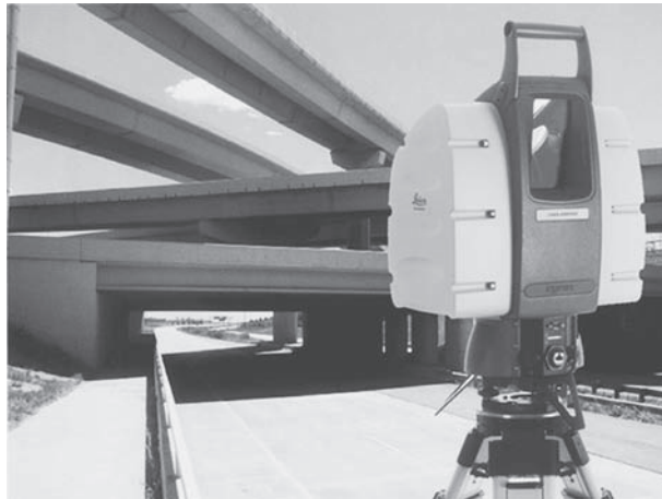
Figure 1.5 LEICA HDS 3000 D24 laser scanner. (Courtesy of Christopher Gibbons, Leica Geosystems AG.)
