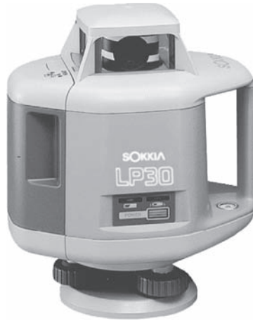
Figure 23.3 Sokkia LP30 laser plane level. (Courtesy Topcon Positioning Systems.)
