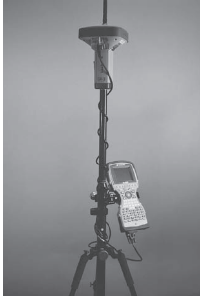
Figure 14.2 A GNSS receiver cabled to survey controller. (Courtesy Topcon Positioning Systems.)
