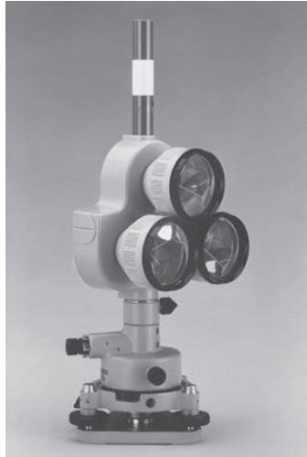
Figure 6.11 Triple retroreflector. (Courtesy Topcon Positioning Systems.)
