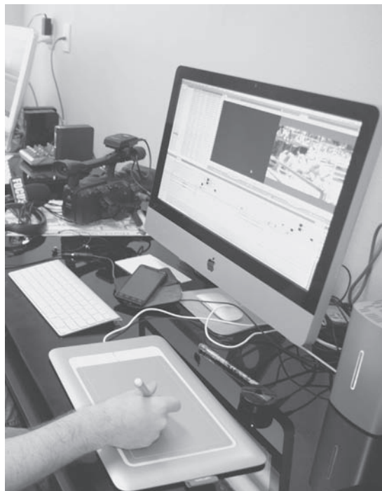
Figure 28.8 Tablet digitizer interfaced with personal computer. (© Jeff Greenberg/ Alamy.)
