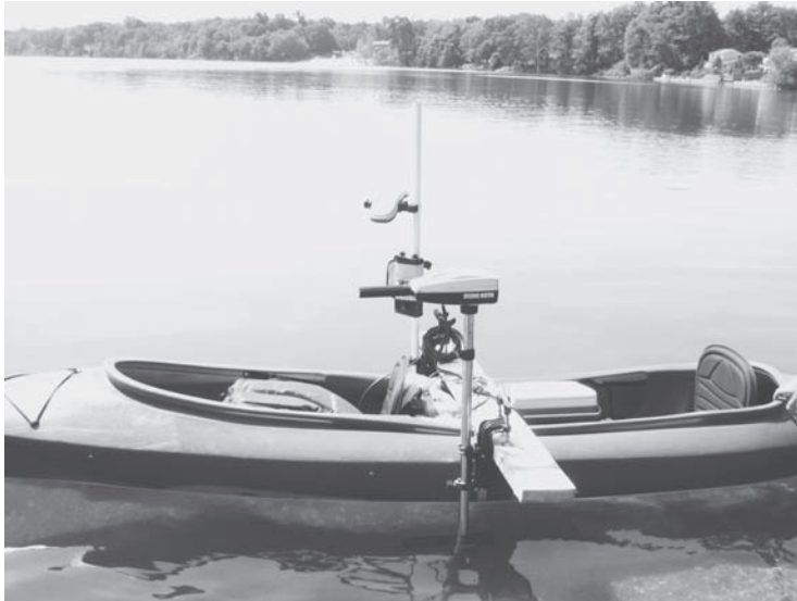
Figure 17.17 Depth sounder used in small lake hydrographic survey. (Sea Floor Systems, Inc.)
