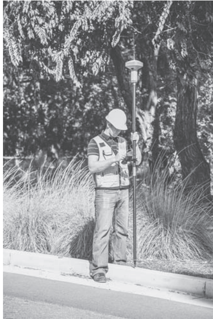
Figure 13.14 The GR-5 receiver is capable of combining GPS and GLONASS signals into a combined solution. (Courtesy Topcon Positioning Systems.)
