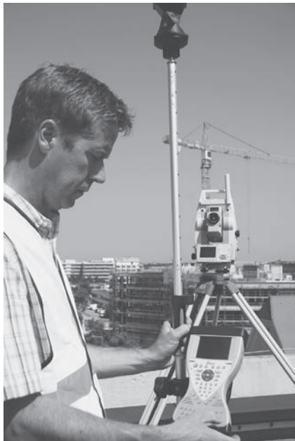
Figure 8.7 A Leica Geosystems robotic total station with its survey controller on the prism pole. (Courtesy Leica Geosystems AG.)
