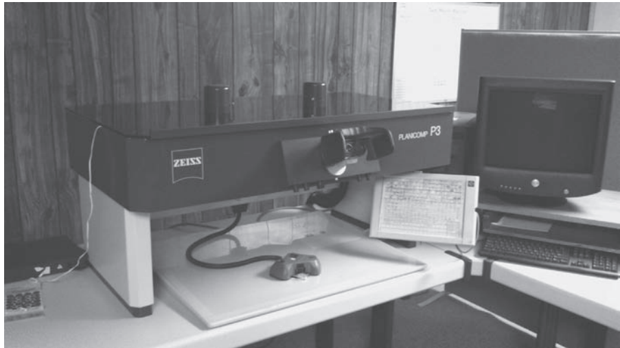
Figure 27.16 Zeiss P3 analytical plotter. (Courtesy Golden Aerial Surveys.)
