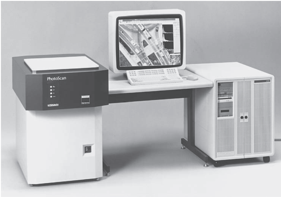
Figure 27.17 Zeiss/Intergraph PS1 PhotoScan. (Courtesy Carl Zeiss.)
