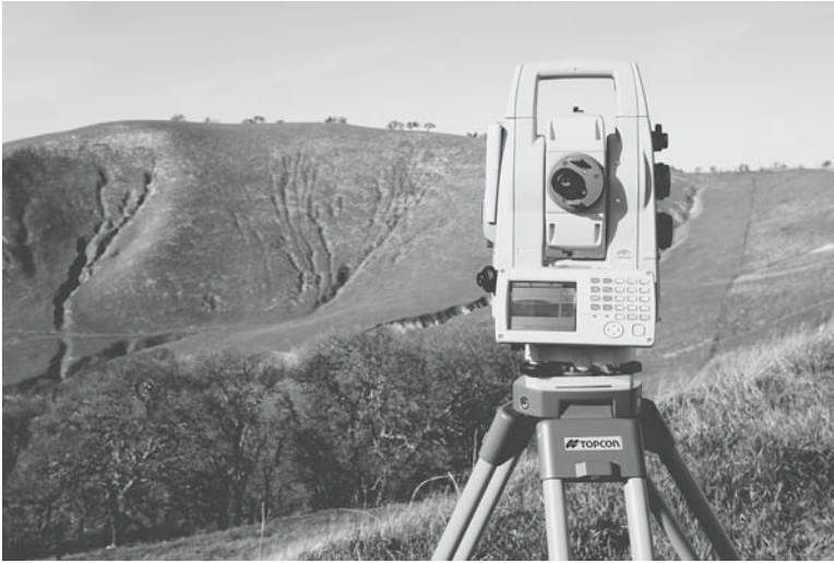
Figure 17.1 Total station capturing image of area to be surveyed. (Courtesy Topcon Positioning Systems.)
