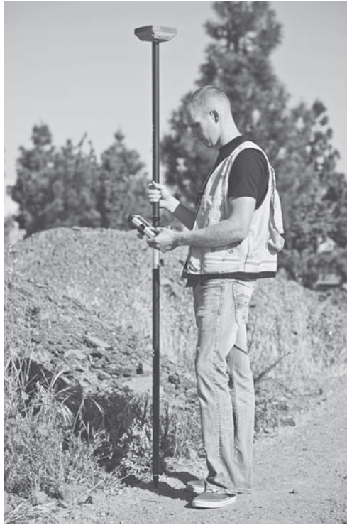
Figure 15.1 The roving receiver being used in a kinematic survey. (Courtesy Topcon Positioning Systems.)
