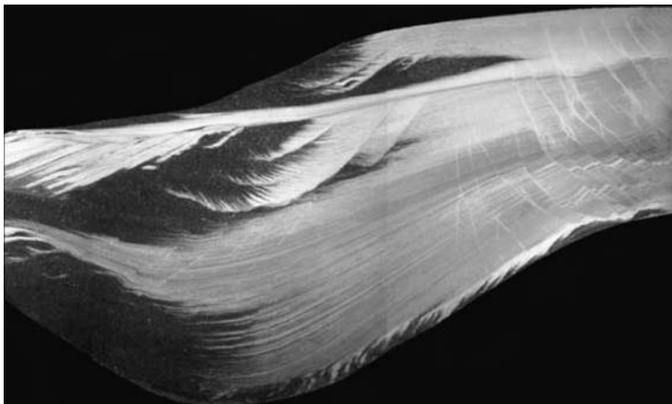
FIGURE 1.2 Experimental results from a subsiding tank, showing the kind of complexity characteristic of deltaic deposits in a subsiding basin. (Reproduced with permission from Paola et al. 2001.)
