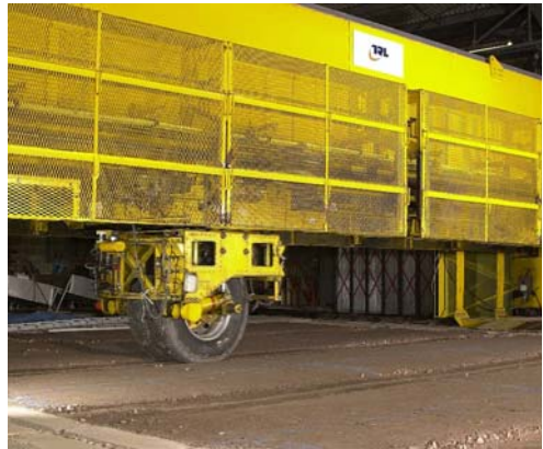
Linear fatigue machine (length 2 m)
