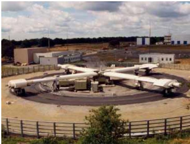
Circular fatigue carousel (diameter 20 m)
