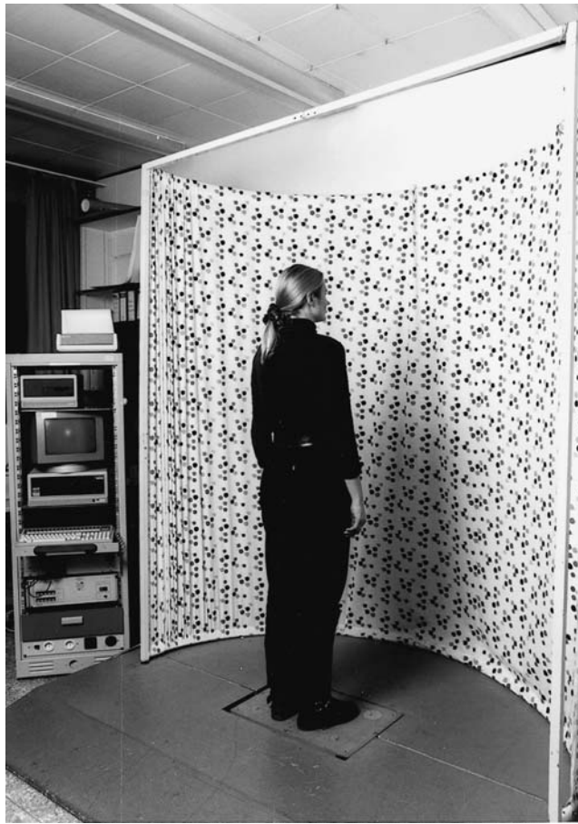
Figure 1.25. Posturography. Posturography allows the examination of control of postural stability (a Kistler platform is used). The parameters include the original registrations of body sway to the right or left, forward or backward, upward or downward; the frequency analysis of the sway (Fourier analysis); and the so-called sway path values (SP, m/min). The SP is defined as the length of the path described by the centre of foot pressure during a given time. Healthy subjects also exhibit body sway as a result of inherent physiological instability when standing on a recording platform; SP is exacerbated in vestibular disorders. The SP values can be derived automatically with a computer for the anteroposterior, mediolateral and craniocaudal directions. These values are calculated as the distances between two consecutive sampling points (measured every 25 ms); the anteroposterior (sagittal = x ) plane, i.e., sagittal sway (calculated as \Sigma|\Delta x| ), the mediolateral (frontal = y ) plane, i.e., frontal sway (calculated as \Sigma|\Delta y| ) and the craniocaudal (transversal = z ) plane, i.e., the transversal sway (calculated as \Sigma|\Delta z| ) or for all three planes as the total SP.
