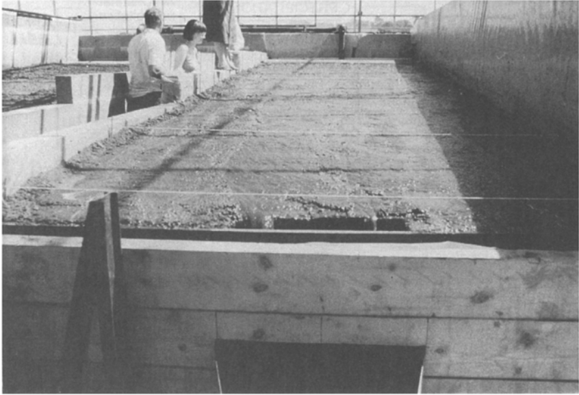
Figure 9.3 A physical model: a soil tank used for analysing overland flow and erosion on semi-arid slope surfaces at the Long Ashton Research Station, University of Bristol, UK. (Photograph courtesy of Professor John Thornes.)
