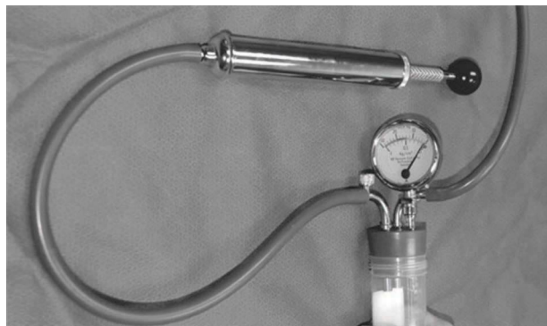
Figure 24.4 The tubing (see Figure 24.3) attaches to one of three fittings on a stopper, which in turn is plugged into a collecting jar. The three metal tubular fittings are as follows: (a) inlet that couples with tubing from the vacuum cup; (b) outlet with vacuum relief valve that couples with tubing leading to the hand vacuum pump; and (c) outlet to the vacuum-recording gauge.
