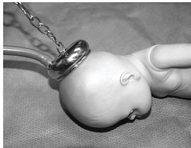
Figure 24.3 The 60-mm (6-cm) vacuum cup is attached to the head of a mannequin. The heavy-gauge tubing (left of image) is attached to a hollow stem on the convex surface of the cup. Traction is applied by the attached traction handle and transmitted to the chain and vacuum cup.
