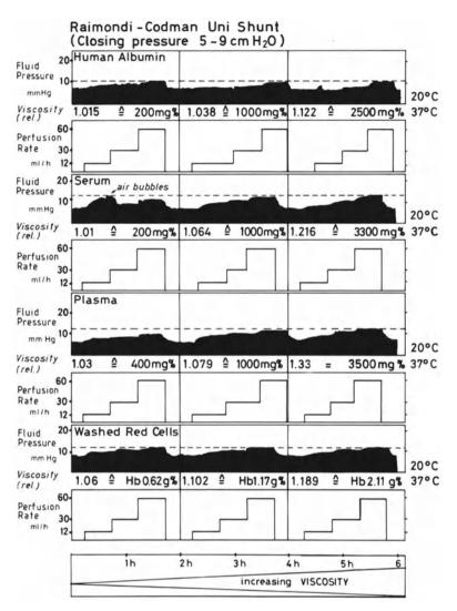
Fig. 3. Influence of VF-viscosity on "ventricular" pressure (balloon pressure) (see Fig. 2), vented by a RAIMONDI one-piece shunt with closing pressure of 5-9 cm  $H_2O$ . Increase of VF-viscosity by admixture of human albumin, serum, plasma, or washed red cells
