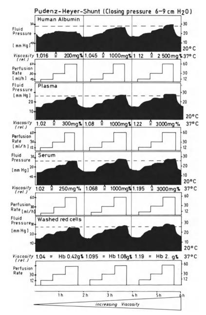
Fig. 4. Influence of VF-viscosity on "ventricular" pressure (balloon pressure) (see Fig. 2), vented by a PUDENZ-HEYER assembly with a closing pressure of 6-9 cm  $H_2O$
