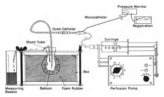
Fig. 2. Influence of VF-viscosity of VF-pressure, examined with the aid of an experimental set-up, consisting of a perfusor, a ventricle-brain-like-model, and a pressure gauge
