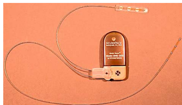
Fig. 1. The implantable Responsive Neuro-Stimulation System (Neuropace, Inc., Mountain View, CA, USA); it is shown in this picture with subdural strip and depth leads
