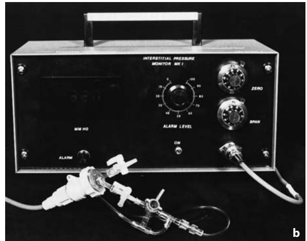
Fig. 20.5a,b. Continuous compartment monitoring. a Position of a slit catheter for measuring compartment pressure. b Measuring device for continuous compartment pressure monitoring. (Courtesy of Dr. Cecil Rorabeck)
