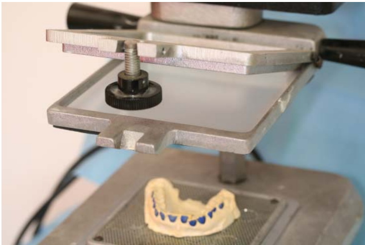
Figure 13.20 Machine loaded with model and tray material
