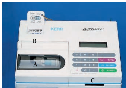
Fig. 8.11 An amalgamator with a capsule of amalgam in position behind a shield (A). The appropriate card is chosen from the rack (B) and inserted into the slot (C). The electronic control is then activated.
