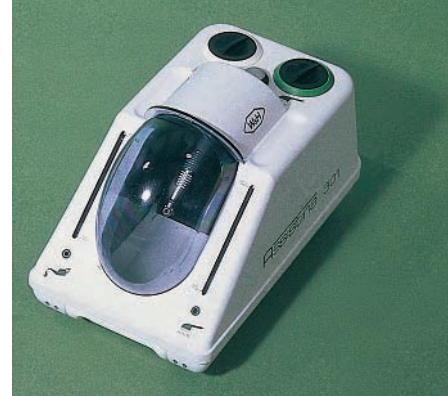
Fig. 5.14 An automatic handpiece cleaning unit which is connected to the air supply. The shield at the front is rotated out of the way and the handpiece plugged onto the connector. A detergent is then flushed through the handpiece followed by oil, both of which come from refillable containers at the back of the unit. This is a more efficient and quicker system than using aerosols.
