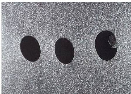
Fig. 4.12 Three holes have been punched in the rubber. The one on the right-hand side has not been cleanly cut and is likely to tear when the rubber is stretched.
