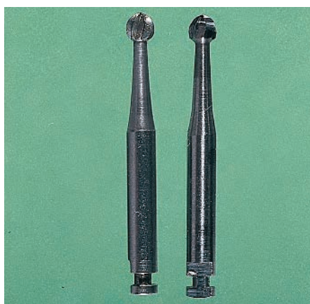
Fig. 5.17 Similar sizes of steel and tungsten carbide burs. The head of the tungsten carbide bur (right) can be seen attached to a steel shank. The head is a slightly different shape.
