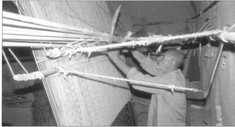
Plate 42 Once the correct pattern cords have been chosen they are pulled forwards and held in place by two large wooden hooks. The rocker system that controls the harness for the structural warps frames the weaver's head. The heddle bars are moved by altering the position of the wooden bar behind his head. The two separate harnesses are clearly visible in Plate 14 .
