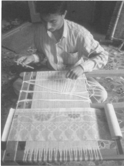
Plate 44 The key operation in drawloom weaving is making the naqsheh , a large-scale version of the pattern to be woven. When complete the 'warp' strings of the naqsheh (draw-cords or simplecords) are attached to the cross-cords on the loom, and the 'wefts' of the naqsheh (lashes) are pulled in sequence by the weaver's assistant, the draw-boy. The pull of the lashes is ultimately transmitted to the warpends on the loom to form the pattern shed. A naqsheh can take weeks to make and demands a high level of skill and concentration (Benares, 1992).
