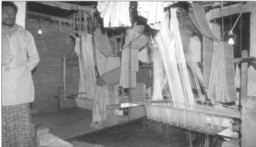
Plate 45 Three naqshehs attached to a loom. The vertical draw-cords are tied to the transverse cross-cords. Below the cross-cords are string heddles which control the warp ends running below and at right angles to the cross-cords. Behind the three naqshehs and running diagonally are three sets of draw-cords belonging to a Jacquard harness which is also being used to weave the same textile. The Jacquard punch cards are on the left (Benares, 1992).
