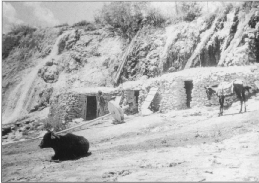
Plate 9 A new millstone for an Afghan mill in Band-e Amir (1977). It is still wedged on the poplar trunk to which the ox in the foreground was harnessed when the stone was trundled here from the quarry. A team of men had urged on the ox and controlled and braked the stone, weighing about one ton, by means of the longer end of the axle.
