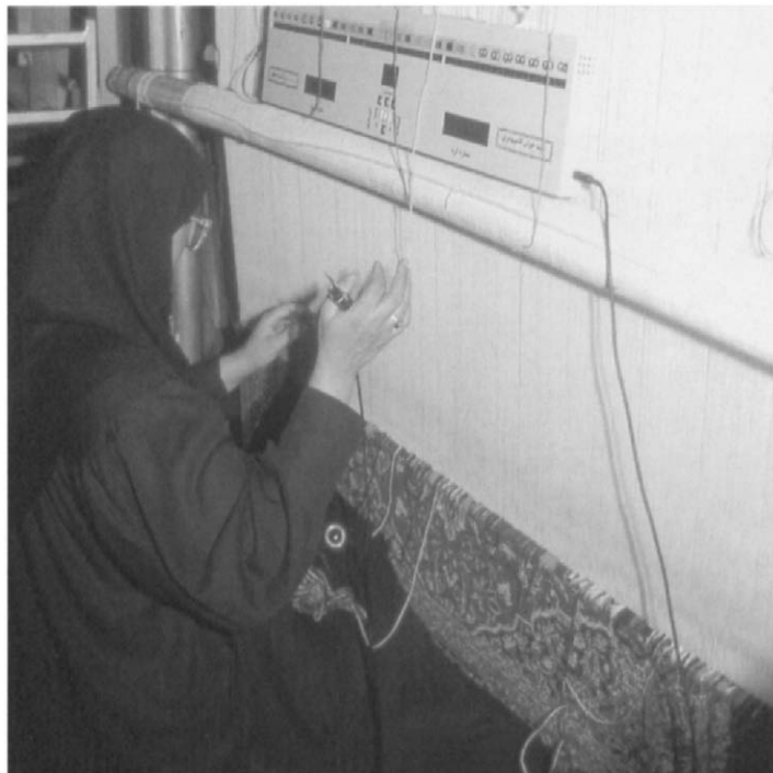
Plate 49 Weaving from an electronic talim . The weaver's instruction is recorded electronically on a memory chip and presented on liquid crystal displays and with coloured lights. After cutting each knot she presses a micro-switch on her knife to update the display. This system avoids the problem of weavers having to find their place every time they refer to the cartoon or talim (Tehran, 1993).
