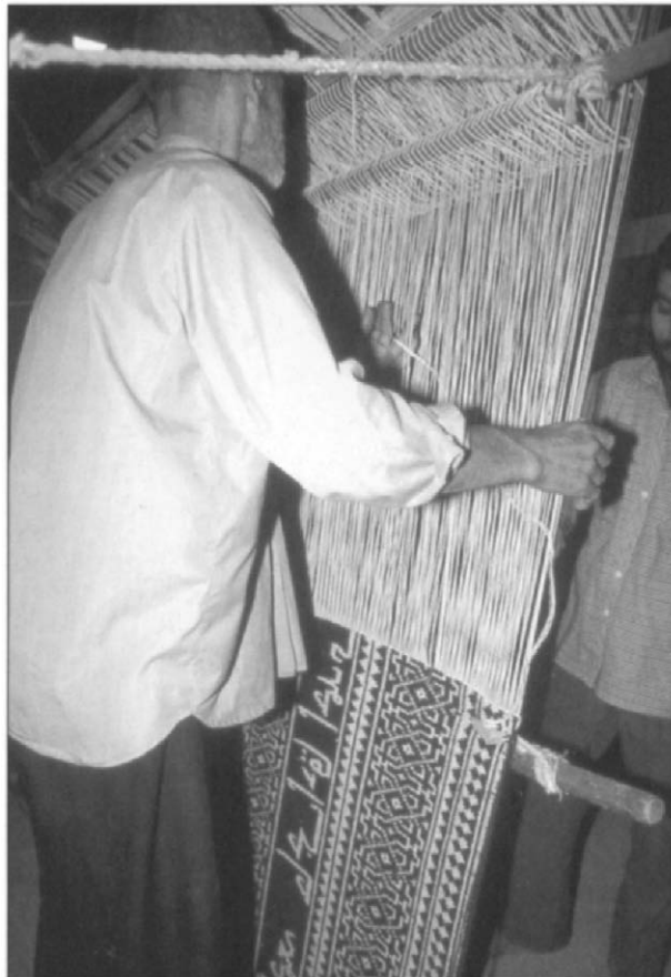
Plate 43 The inscription is woven 'freehand'. The weaver manipulates the 19 pattern cords as he goes along. Inscription bands (other than such motifs as repeating kufesque forms at the top of the field) always run in the warp direction. Thus the saf shown in Plate 39 has 16 niches side by side in two rows, a common arrangement, whereas others would have had many rows, perhaps four niches across (Meybod, 1984).
