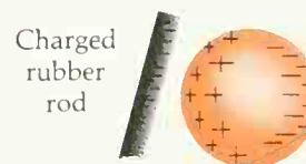
(b) A negatively charged rod is brought near the sphere, repelling some electrons (which move freely in the metal) to the opposite side, leaving positive charges near the rod.
