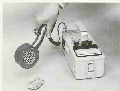
(b) A portable battery-operated Geiger counter measures the activity of pitchblende, a radioactive mineral containing uranium.
