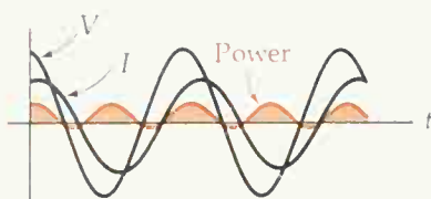
(b) An inductive reactance with resistance. The current I lags the applied voltage V : \phi = 45^\circ . When the power is negative, energy is being returned from the inductance to the source.
