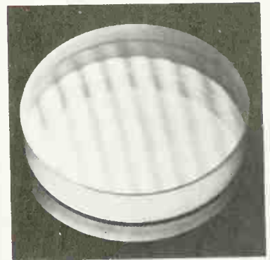
(b) The surfaces are in contact at one edge and separated a small amount at the opposite edge. The regularly spaced bright and dark fringes indicate that the surface is uniformly flat.
