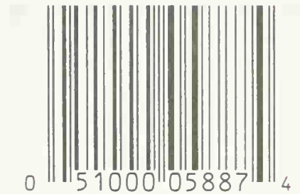
FIGURE 44-18 The bar code scanner in supermarket checkout counters uses a narrow beam from a He-Ne laser to sweep across the Universal Product Code (UPC) symbol that identifies the item. The reflection from the light and dark bars is detected by a photocell, and the information is sent to a central computer. If the number is listed in the computer memory, the scanner sounds a beep, prints out the product information and price on the sales slip, and tallies the sale of that item in the store's inventory records. Some stores analyze daily records to make smart marketing decisions, taking advantage, for example, of the evidence that candy bar sales zoom when the bars are placed near the checkout counter, or that sales of bean dip increase if taco chips are on sale. Daily record analysis can also measure the effectiveness of a newspaper advertisement vs. an in-store display. In the code above, the initial zero identifies a grocery item, the next five digits the manufacturer (The Campbell Soup Co.), the next five digits the specific item (10 \frac{3}{4} oz., reduced-salt, condensed tomato soup), and the final digit the weight or volume.
