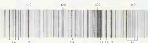
(b) A segment of the visible spectrum of the sun. Wavelengths (in nanometers) are listed above the spectrum, while elements responsible for certain strong lines are shown below.
