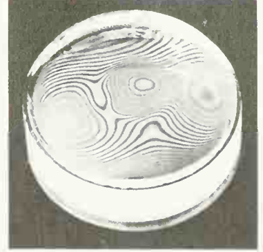
(a) A wavy fringe pattern indicates an uneven surface. Three "high" (or "low") spots are revealed by the regions of circular fringes.
