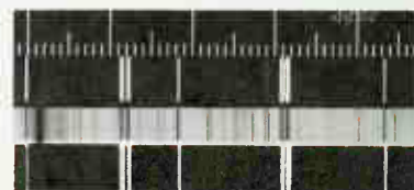
(c) A laboratory (bright-line) spectrum of iron is placed above and below the sun's absorption spectrum for comparison, indicating the presence of iron in the sun.
