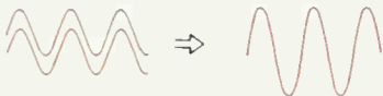
(c) Two light waves in phase superpose to produce an extra bright light (increased intensity). This is called constructive interference .
