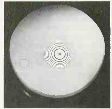
(b) Photograph of Newton's rings obtained with monochromatic light.
