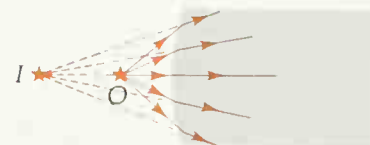
(c) If the refraction is insufficient to produce converging rays, a virtual image is formed outside the medium. (Of course, only an observer within the medium could intercept the rays after they have been affected by the interface, and thus see the virtual image.)
