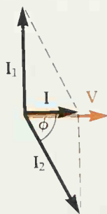
(b) The current phasor diagram at resonance.
