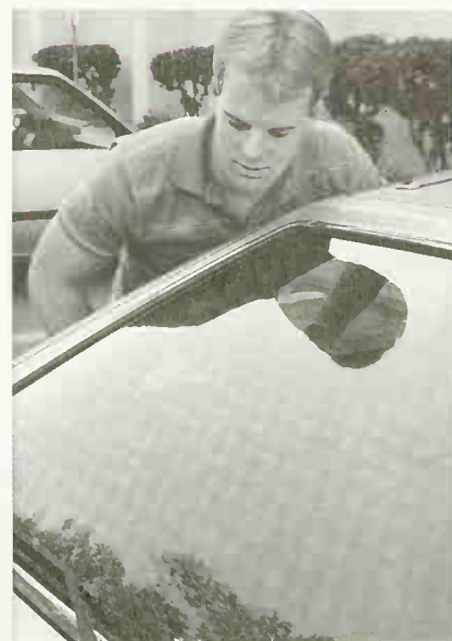
FIGURE 40-10 Safety glass used for the front windshields of automobiles is usually formed of a transparent plastic sheet glued between two glass sheets so that if the windows shatter the glass fragments will be held together. The side and rear windows, however, are often a single sheet of glass heat-treated in a way that purposely introduces mechanical strains into the glass as it cools. If broken, the entire window then crumbles into relatively safe, gravel-sized fragments rather than shattering into large shards as ordinary glass does. The strains make the glass birefringent. As shown here, you can see this strain pattern when partially polarized sky light is reflected at the Brewster angle from the rear window. Although no polarizing filters were used for this photograph, viewing the reflection with polarizing sunglasses makes the strain pattern even more pronounced.
