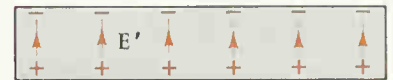
(b) The induced field E' due to the induced charges on the surface of the dielectric material when it is placed between the plates. (Plates are not shown.) Note the direction of the field E' .
