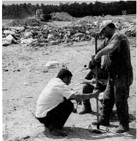
Figure 4 Dynamic penetrometer tests
