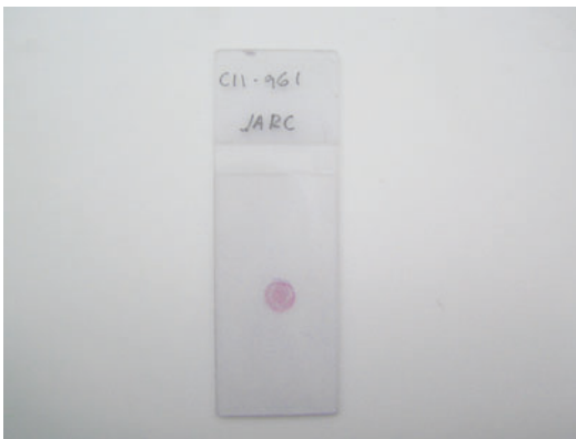
Cytospin Technique, Fig. 3 The final monolayer slide with the material consistent with a clearly defined 6 mm area
