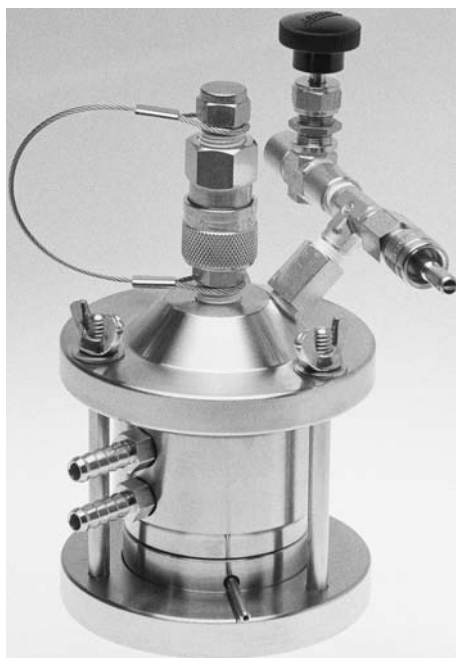
Figure 1 A research scale extrusion device (Lipex™ Extruder) manufactured by Northern Lipids (Vancouver, BC, Canada) has a 10-mL capacity and can be operated over a wide range of temperatures when used in combination with a circulating water bath. The quick-release sample port at the top of the unit allows for the rapid cycling of sample through the filters.
