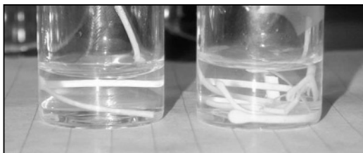
Figure 8. Epoxy gel strips without (left) and with immobilized alkaline phosphatase after immersion in p-nitrophenylphosphate. Both the gel and solution on the right become yellow due to the action of the enzyme to form p-nitrophenol.
