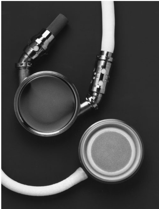
Figure 67-3. The textured internal surfaces of the Heartmate left ventricular assist device. (Courtesy of Thoratec Corp., used with permission.)
