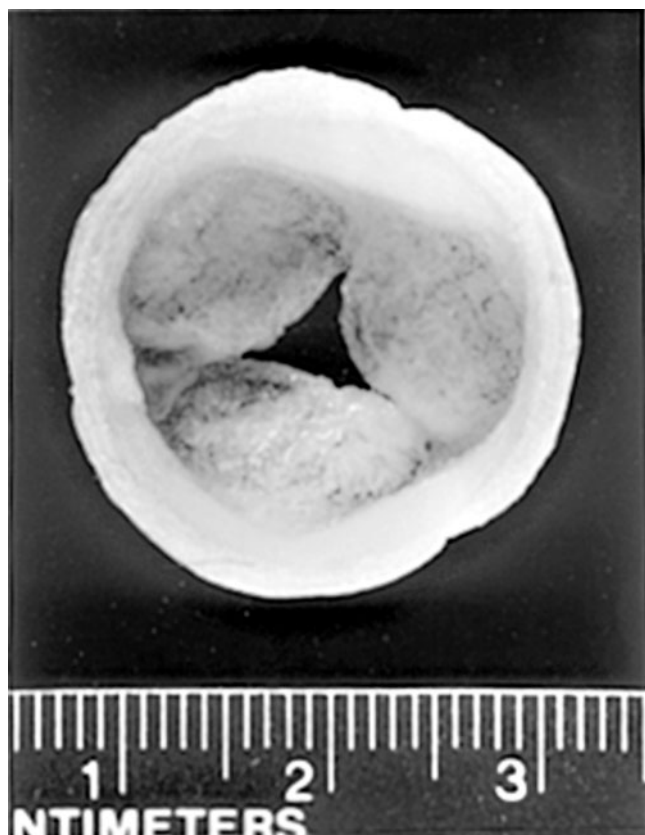
Figure 5-10. Tissue engineered heart valve composed of ovine vascular wall cells seeded on polyglycolic acid polymer scaffold and conditioned in a pulsatile bioreactor in vitro for 14 days. (Reproduced with permission from Hoerstrup et al. 91 )
