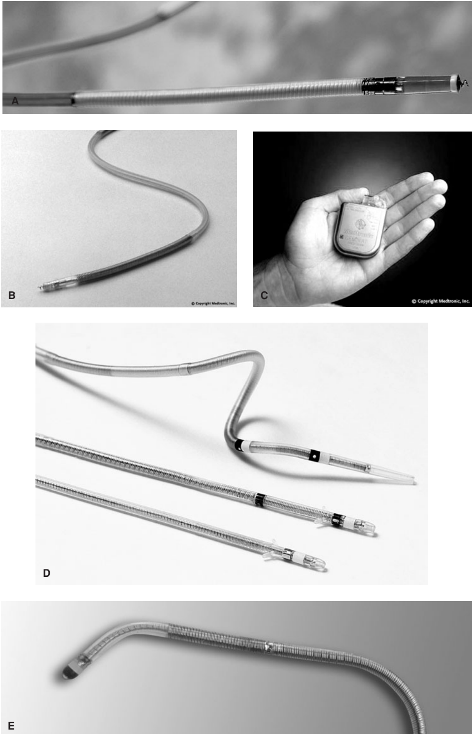
Figure 60-27. (A) Recent 9F ICD lead with Gore-Tex-coated shocking coils. (B) Recent 7F ICD lead with retractable screw. (C) Recent ICD/pacemaker. (D) Recent over-the-wire leads for coronary sinus pacing. (E) Recent over-the-wire lead for coronary sinus pacing. (A and D: Courtesy Guidant Corp., Indianapolis, Ind; B, C, and E: Courtesy of Medtronic, Inc., Minneapolis, Minn.)
