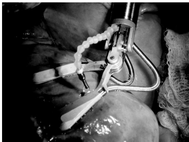
Figure 26-6. Endoscopic coronary artery bypass grafting. New endoscopic vacuum stabilizer including irrigating channel. The stabilizer is mounted to the fourth arm of the new da Vinci system and can be operated remotely by the surgeon at the console.
