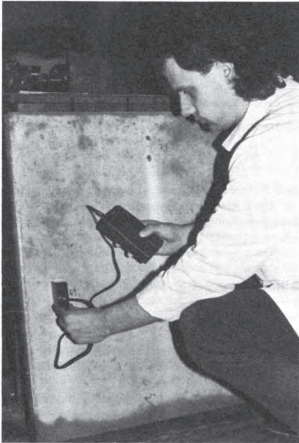
Fig. 5.2 A resistivity meter developed for concrete.
