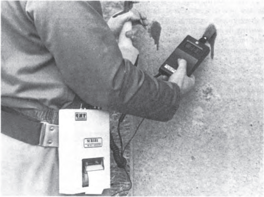
Fig. 5.3 Potential measurement and logging (courtesy of CMT Ltd, Raynesbury, Derby)
