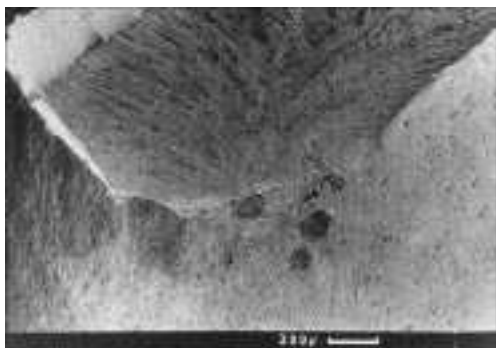
6.2 Brittle fracture as a result of chloride-assisted corrosion attack.
