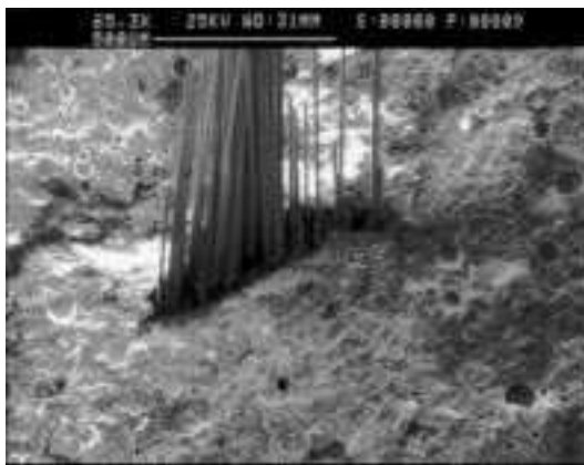
9.11 Microstructure of sulpho-aluminate modified glass-frc, SEM of aged (28 days at 65°C) fracture surface showing pseudo-ductile 'telescopic pullout'.
