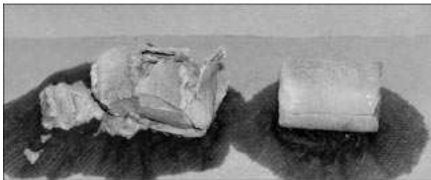
4.2 Thaumasite sulfate attack in SRPC/powdered limestone paste specimen exposed to \text{MgSO}_4 solution for 100 days at 5^\circ\text{C} (LHS) and absence of attack on similar specimen exposed at 20^\circ\text{C} (RHS).
