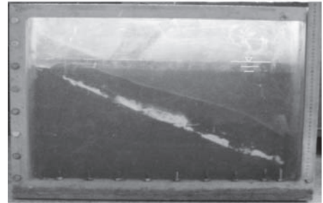
Figure 3. Centrifuge model failed at an acceleration of 10 g.
