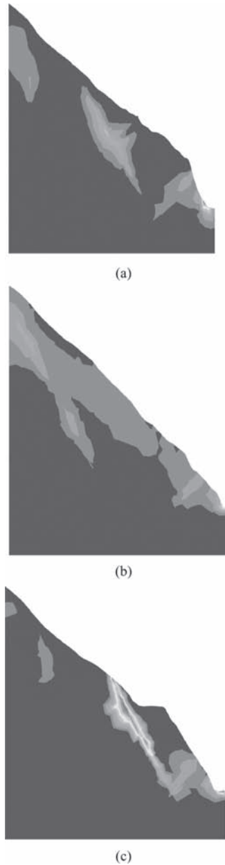
Figure 8. Slope failure modes in different cross sections by numerical modeling.
