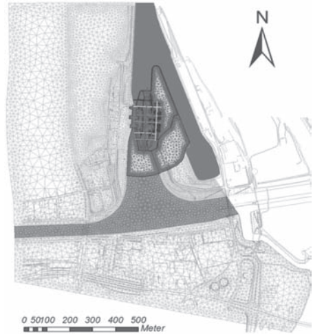
Figure 7. 2D-large-scale model (green) and the 3D-model (red). Lines in the area of the excavation pit: calculation sections.
