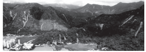
Figure 11. Natural terrain landslides at Tung Chung, Lantau Island during the June 2008 rainstorm.
