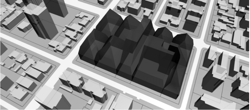
Figure 3: Volumes defined by the front yard regulation ( Antejardin ) for each property fusion.
