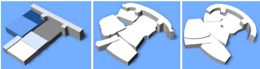
Figure 1: Steps of the morphing procedure. Left: start shape with functional parallelepipeds. Center: intermediate configuration created by the morphing software. Right: final ideal shape from the original project.
