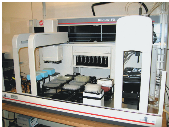
Fig. 4.2 Beckman-Coulter dual-bridge robot equipped with span-8 and 96-pipettor units, a vacuum manifold used for filtering 96-well plates, and an orbital mixing unit
