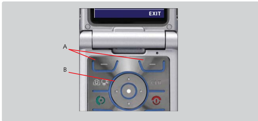
Figure 5.18: The left and right soft keys (A) and the five-way navigation buttons (B).
