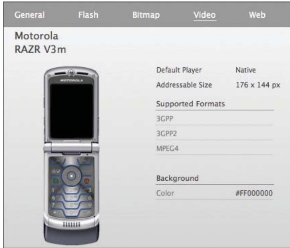
Figure 10.2: Click the Video tab to see which formats are supported by a device.
