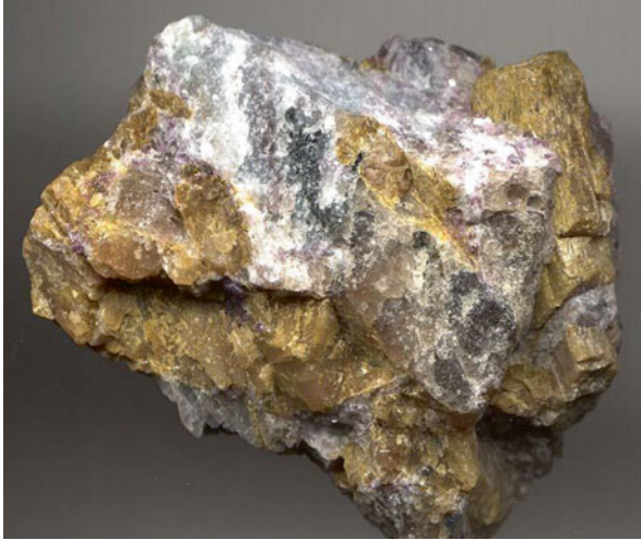
Fig 3.1 Spodumene—a pyroxene mineral consisting of lithium aluminum inosilicate, \text{LiAl}(\text{SiO}_3)_2 , a source of lithium
