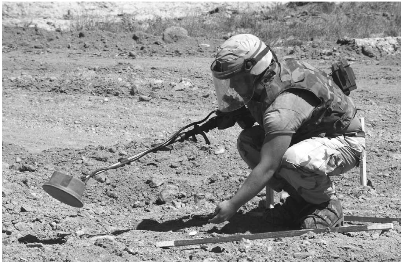
A soldier from the U.S. Army 41st Engineer Battalion uses a metal detector to mark land mines and unexploded ordnance near Bagram Air Base in Afghanistan, 2004. (U.S. Department of Defense)
