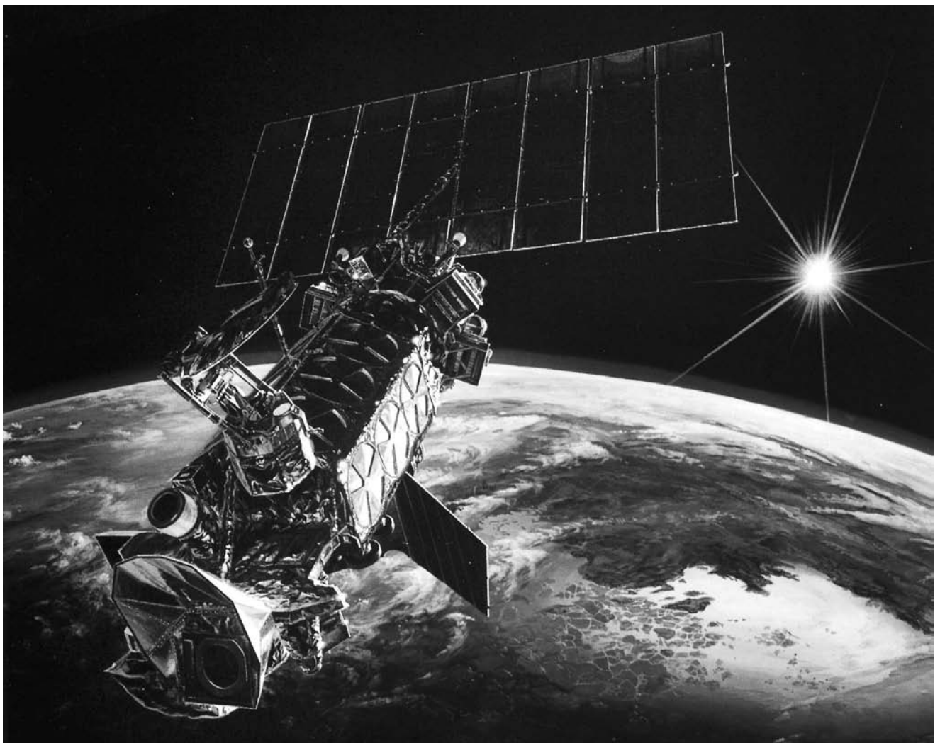
An illustration of a Defense Satellite Communications System (DSCS) satellite. (U.S. Air Force)
