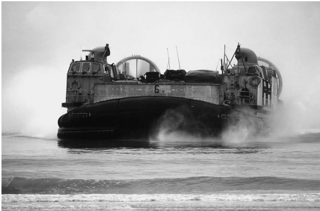
Landing Craft Air Cushion (LCAC) vehicles are hovercraft employed in amphibious landing operations. (U.S. Department of Defense)
