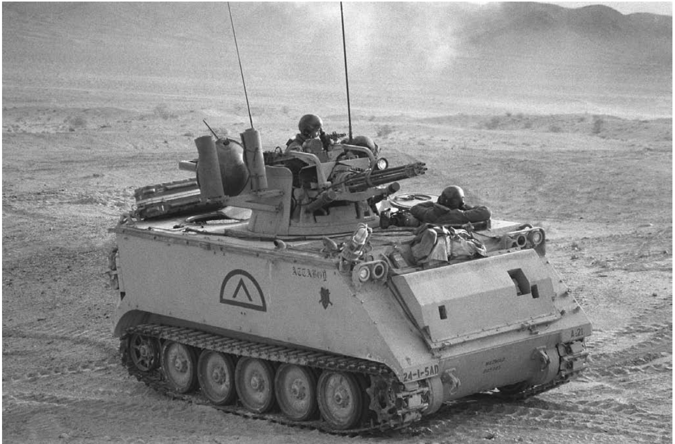
A U.S. Army M163 Vulcan self-propelled anti-aircraft gun system. (U.S. Department of Defense)
