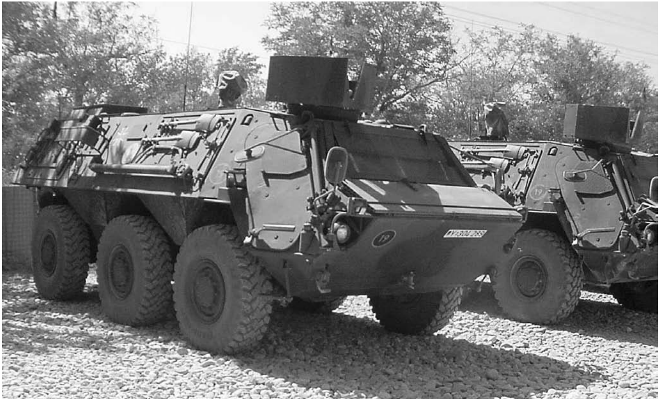
The Fuchs (Fox) M93 NBC Vehicle. Built in Germany, both the United States and Great Britain purchased the Fuchs, which is used to test for nuclear, biological, and chemical contamination on the battlefield. (U.S. Department of Defense)
