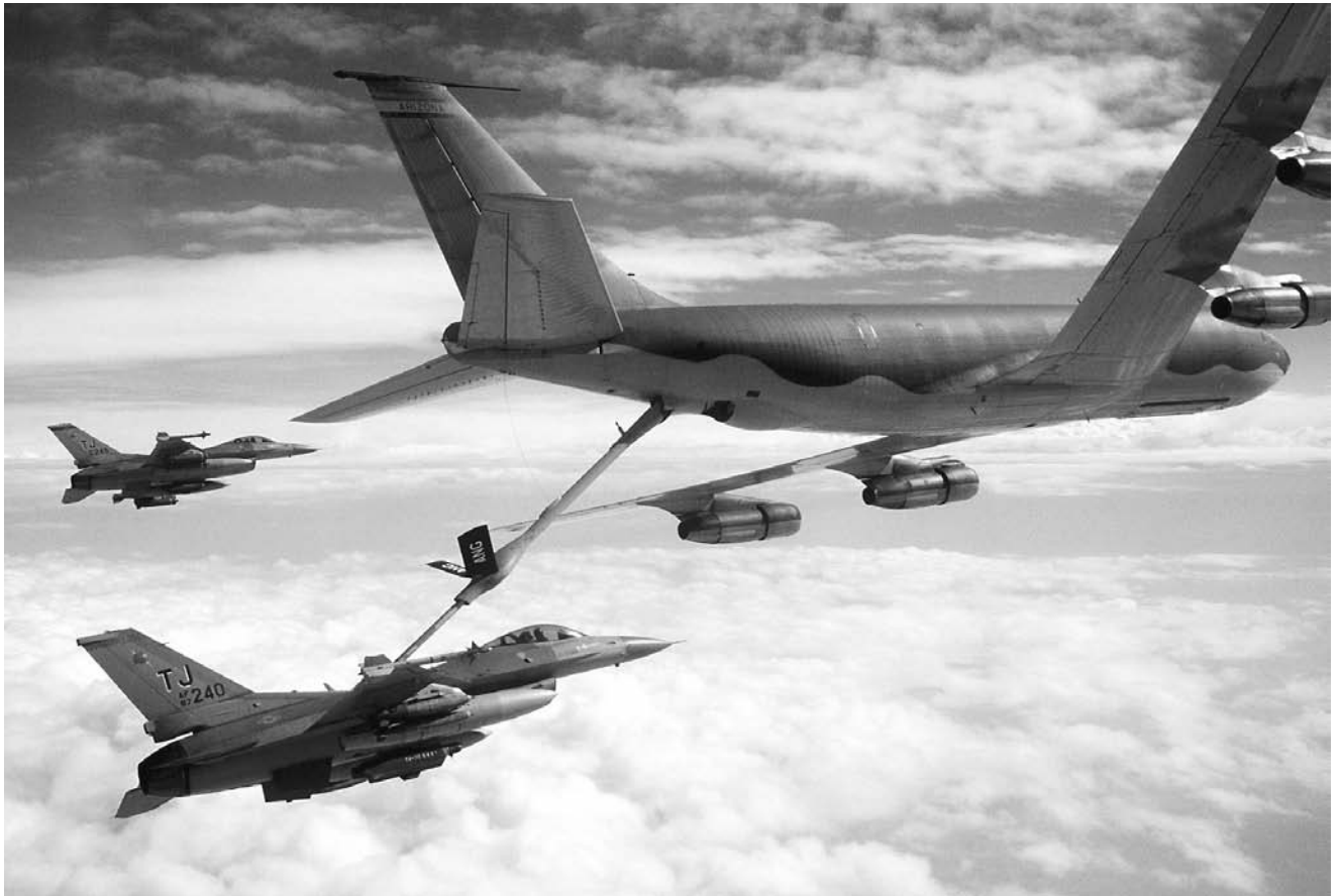
A U.S. Air Force 401st Tactical Fighter Wing F-16C Fighting Falcon aircraft refuels from a KC-135 Stratotanker aircraft as another F-16 stands by during Operation DESERT STORM. (U.S. Department of Defense)
