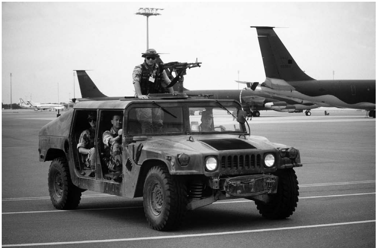
Members of the U.S. Air Force 170th Security Police Squadron patrol an air base flight line in an M998 High Mobility Multipurpose Wheeled Vehicle (Humvee) mounting an M-60 machine gun during Operation DESERT STORM. (U.S. Department of Defense)
