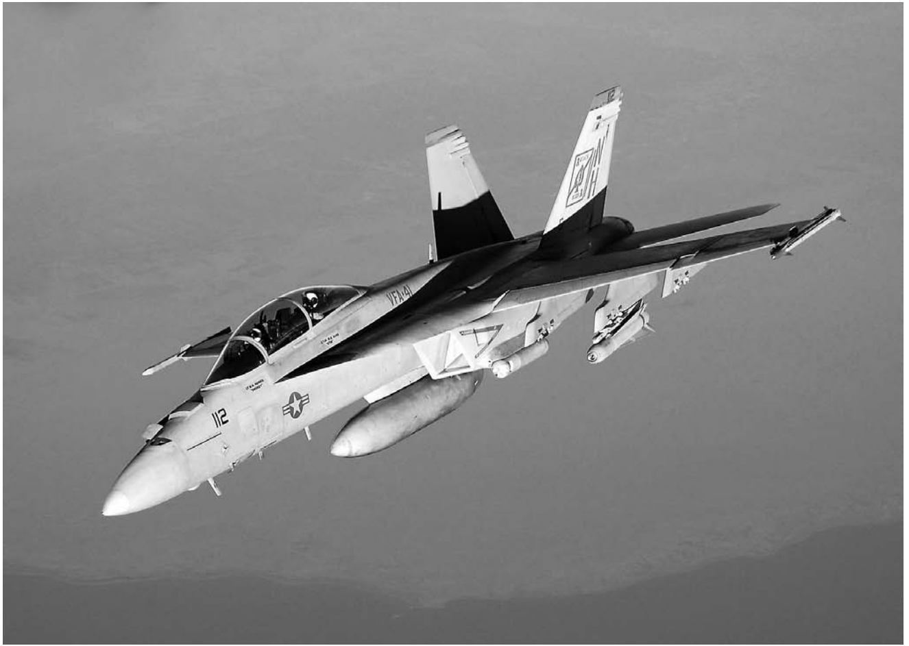
A U.S. Navy F/A-18F Super Hornet conducts a mission over the Persian Gulf in 2005. The Hornet is armed with an AIM-9 Sidewinder missile on the wingtip and an AGM-65 Maverick missile on the pylon. Tucked under the intake is an AAQ-14 LANTIRN (Low-Altitude Navigation and Targeting Infrared for Night) pod. (U.S. Department of Defense)
