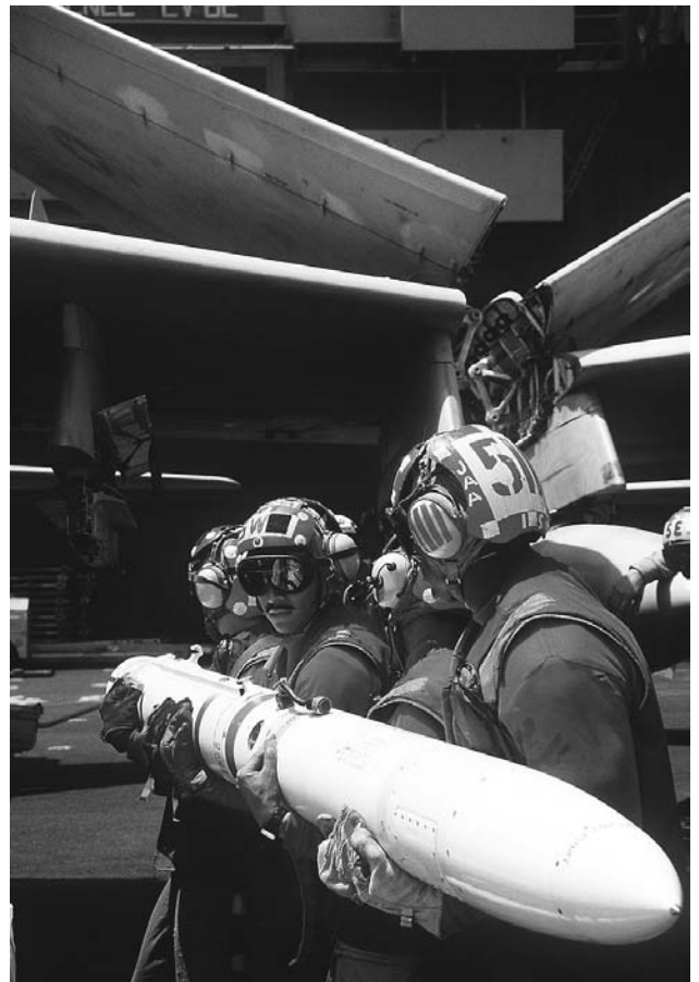
Aviation ordnancemen carry an AGM-88 High-Speed Anti-Radiation Missile (HARM) to an aircraft on the flight deck of the U.S. aircraft carrier Independence . The AGM-88 HARM is an air-to-surface missile designed to seek out and destroy enemy radar-equipped air defense systems. (U.S. Department of Defense)
