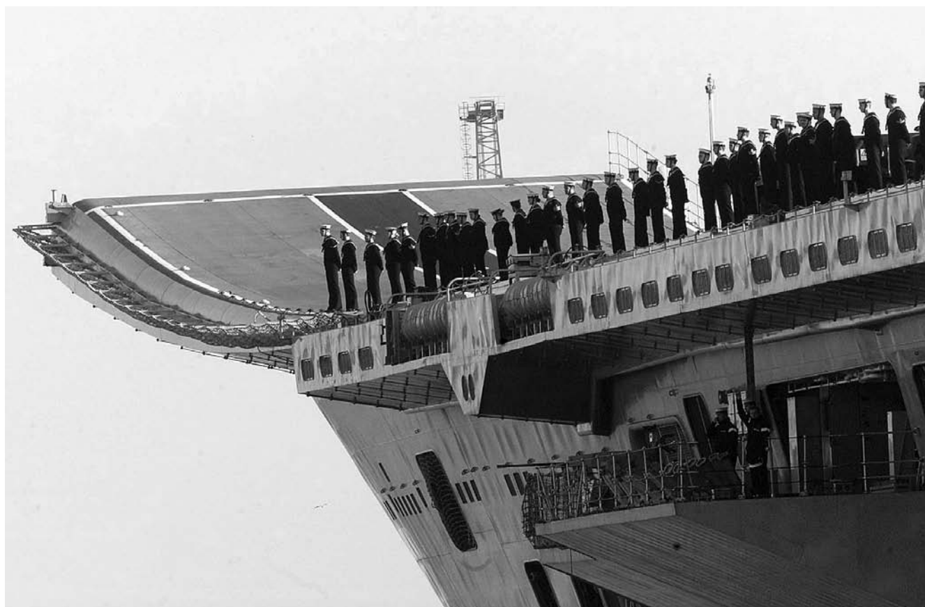
The British light aircraft carrier Ark Royal . Note the 12-degree ski-jump ramp forward to improve take off performance of its Harrier aircraft. (AP/Wide World Photos)
