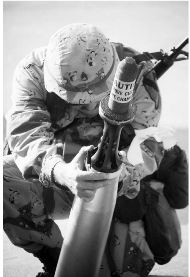
An ammunition specialist examines a 105-mm armor-piercing sabot round to be used in an M-1 Abrams main battle tank during Operation DESERT STORM. Many antitank projectiles contain depleted uranium, but the U.S. Department of Veterans Affairs holds that there is little reason to believe that depleted uranium played a role in causing Gulf War Syndrome. (U.S. Department of Defense)
