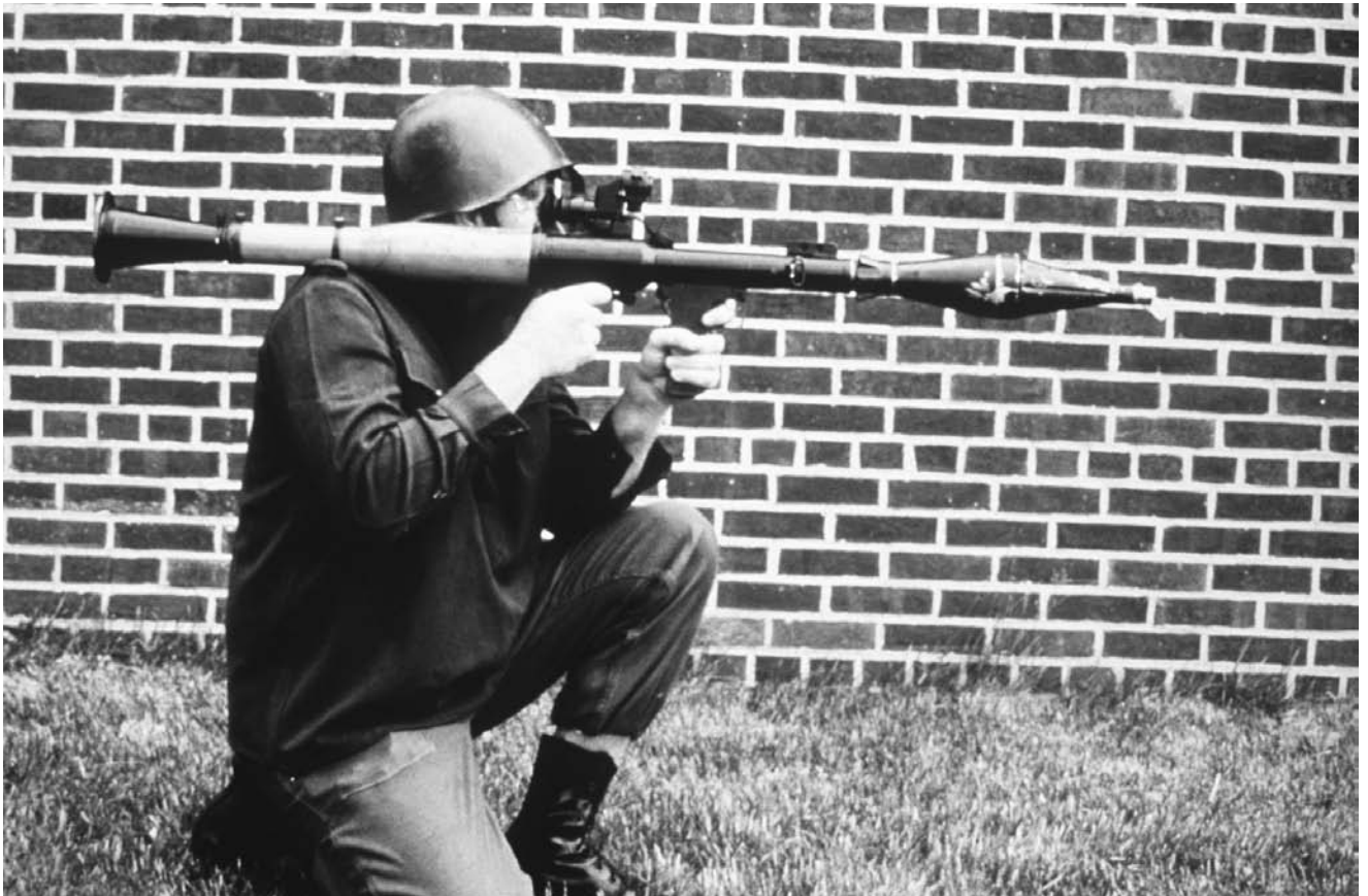
Demonstration of a Soviet-made RPG-7 portable antitank rocket launcher, similar to those employed by Iraqi forces in the Persian Gulf and Iraq wars. (U.S. Department of Defense)
