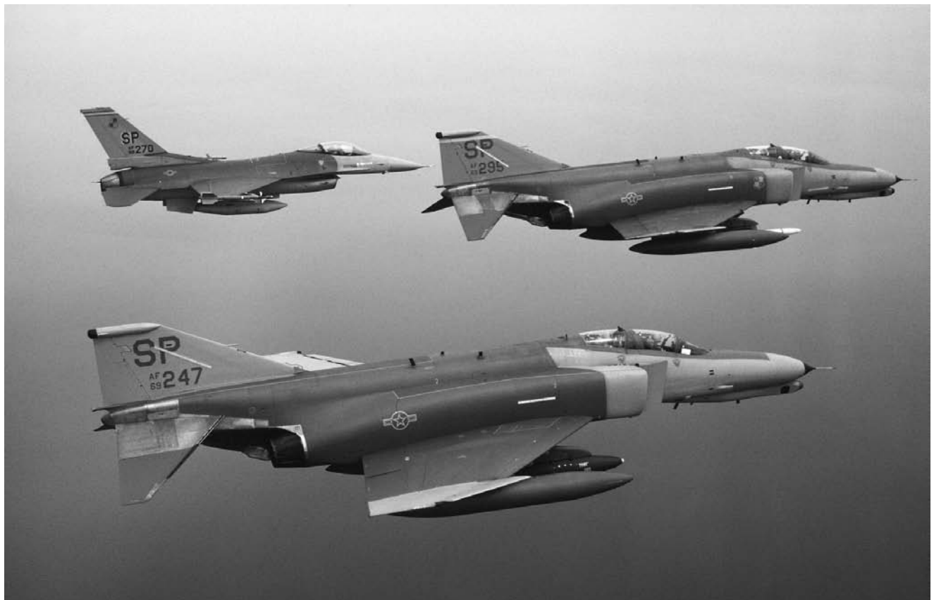
An F-16C Fighting Falcon “Wild Weasel” aircraft, top left, and two F-4G Phantom II “Wild Weasel” aircraft from the U.S. Air Force 81st Tactical Fighter Squadron, 52nd Tactical Fighter Wing. The Fighting Falcon is armed with AIM-9 Sidewinder missiles and the lead Phantom II with an AGM-88 high-speed antiradiation missile (HARM). (U.S. Department of Defense)
