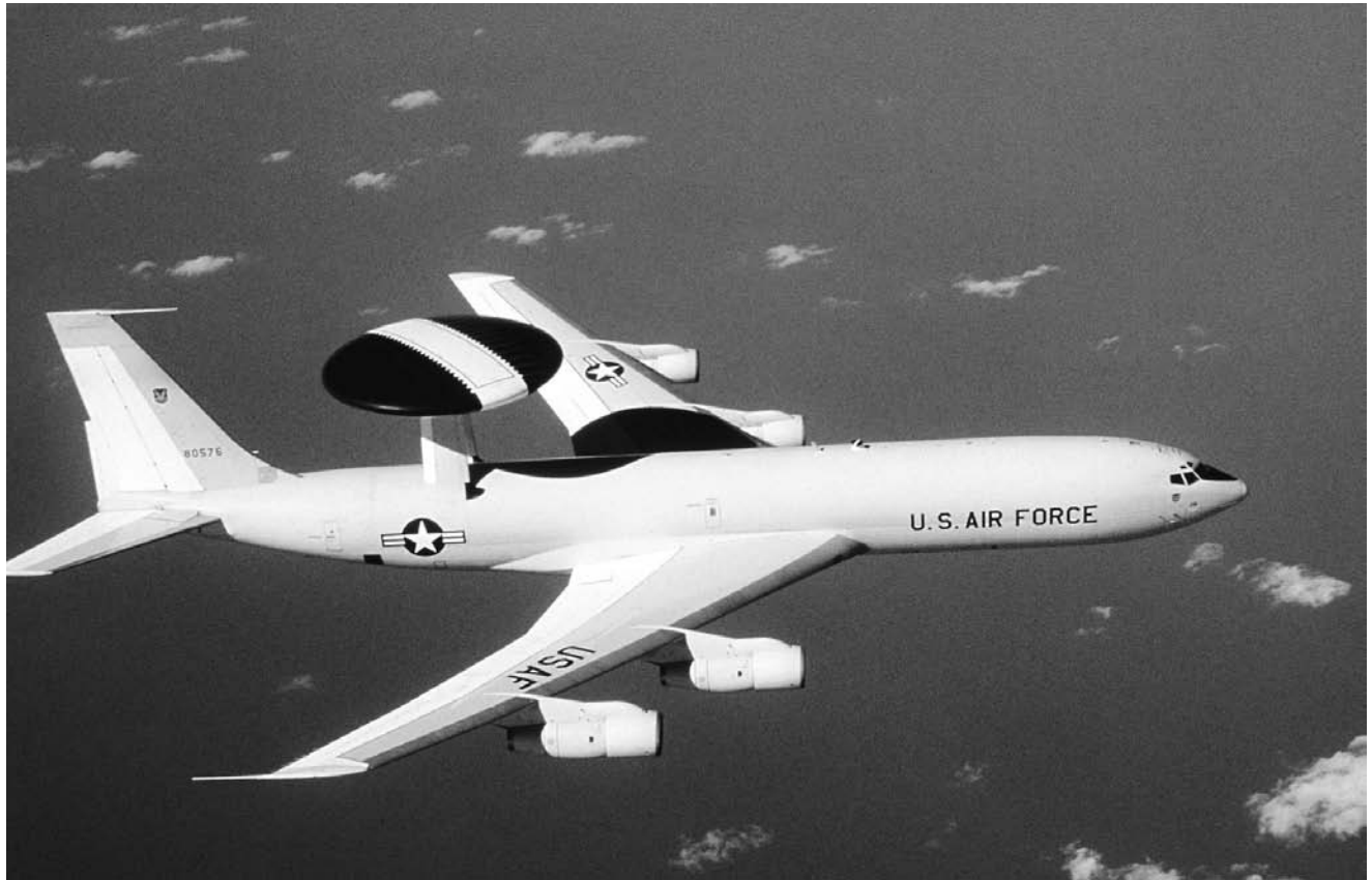
The E-3 Sentry Air Warning and Control System (AWACS) can detect, identify, and track enemy aircraft from great distances and direct fighter-interceptor aircraft to the enemy targets. AWACS has been a critical tool for allied forces during the U.S. wars in the Middle East. (U.S. Department of Defense)
