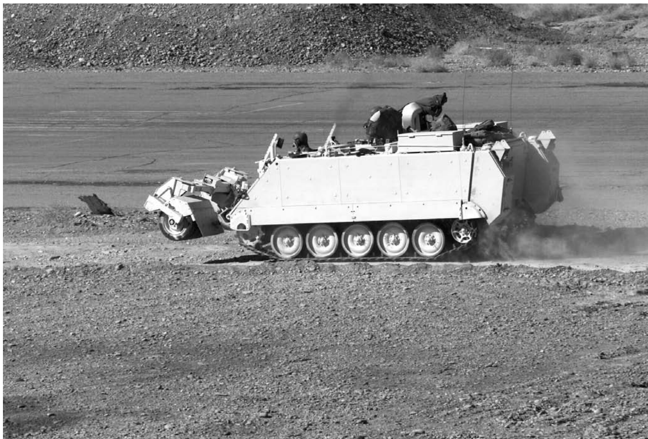
A Norwegian M-113 armored personnel carrier, equipped with a mine roller in front, drives along the runway at Kandahar International Airport, Kandahar, Afghanistan, during Operation ENDURING FREEDOM in 2002. (U.S. Department of Defense)
