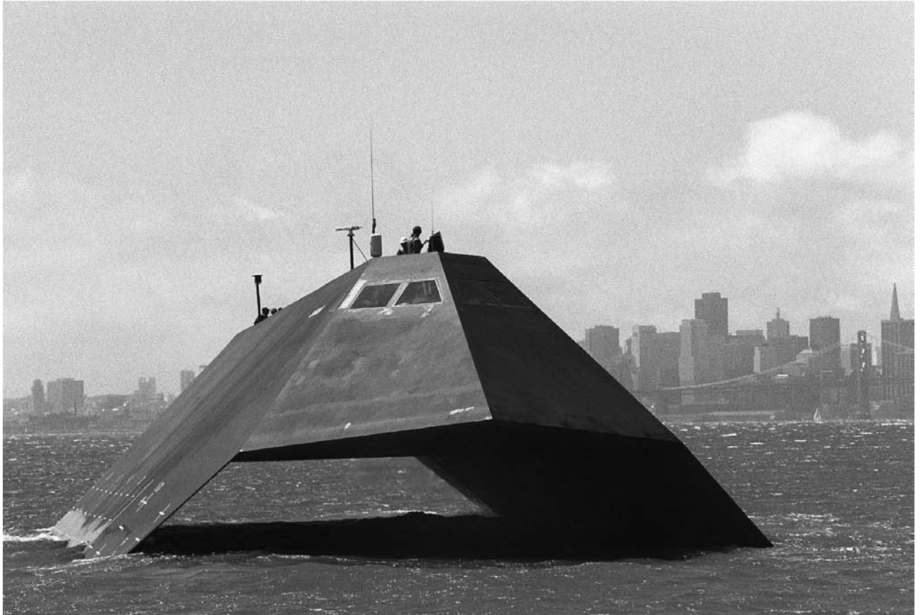
A bow view of the experimental stealth ship Sea Shadow underway in San Francisco Bay, 1993. (U.S. Department of Defense)
