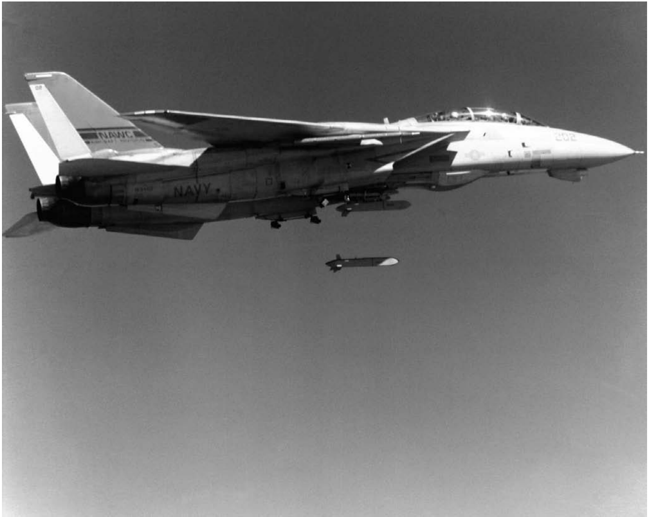
A U.S. Navy Grumman F-14 Tomcat is shown conducting a separation test of the tactical air-launched decoy (TALD), 1994. (U.S. Department of Defense)
