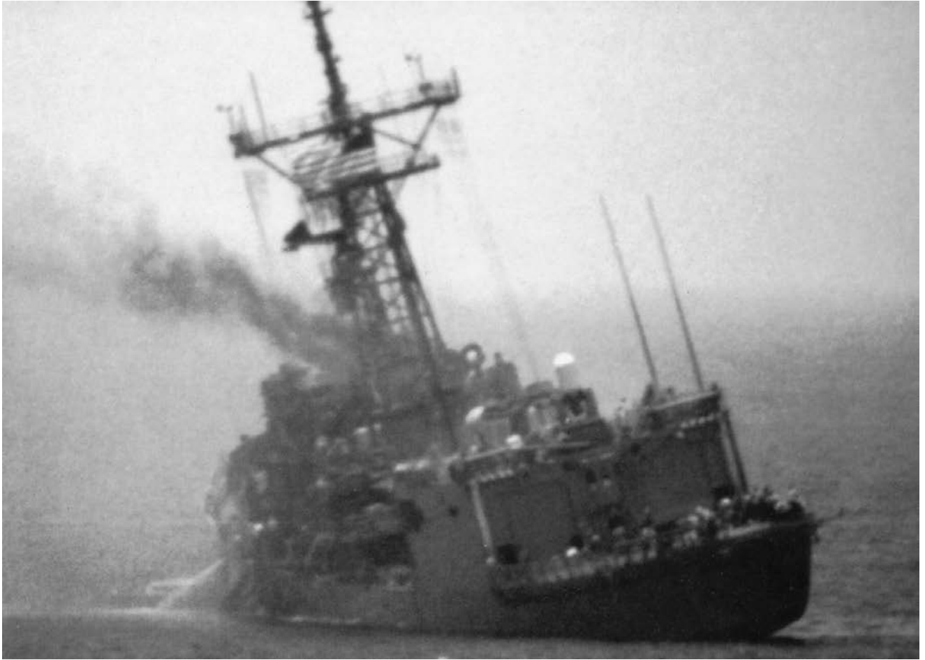
The U.S. Navy guided-missile frigate Stark limps to port after being hit by two Iraqi-fired Exocet air-to-surface missiles. The ongoing hostilities between Iran and Iraq affected other nations in the Persian Gulf region, and the U.S. Navy provided a measure of stability and protection to international shipping there, although not without price. (Naval Historical Center)
