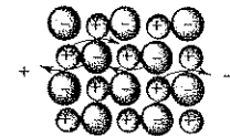
Figure 2.10 When voltage is applied to an ionic material, entire ions must move to cause a current to flow. Ion movement is slow and the electrical conductivity is poor.
