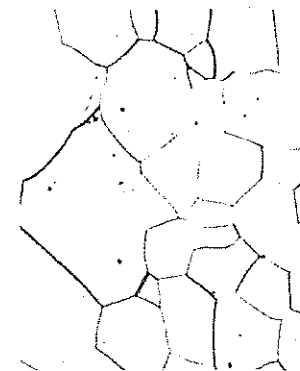
Figure 4.16 Microstructure of palladium, ( \times 100 ). (From Metals Handbook, Vol. 9, 9th Ed., American Society for Metals, 1985.)
