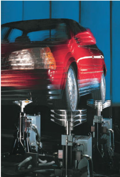
An automobile undergoing vibration testing of its suspension system.
