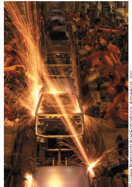
Robots welding automobile unit-bodies.
