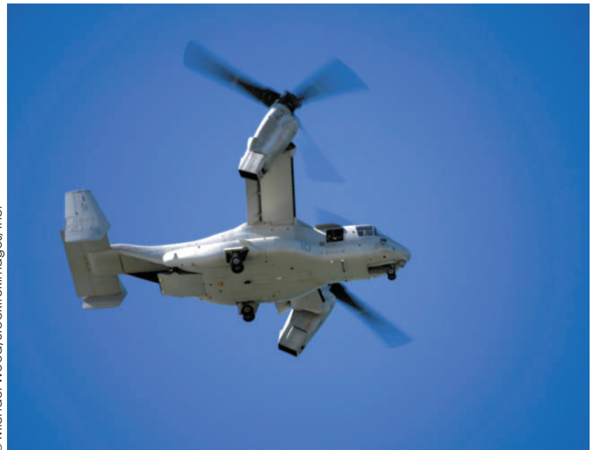
The engine/propeller units at the wingtips of this aircraft can tilt from a vertical takeoff position to a horizontal position for forward flight.
