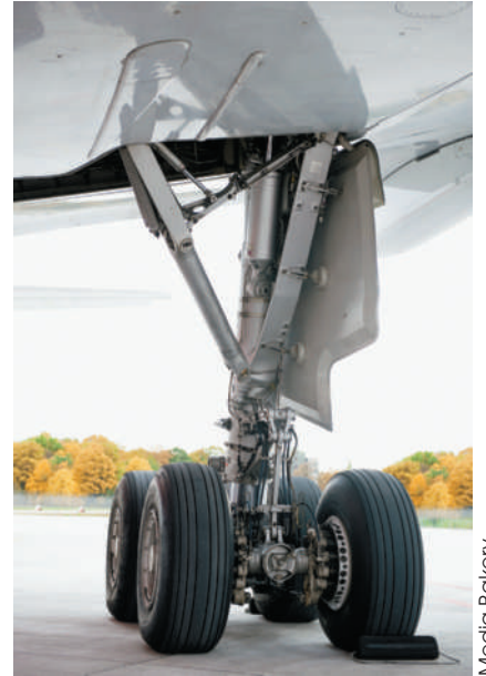
Portions of the landing gear for a large aircraft undergo three-dimensional motion during retraction and deployment.
